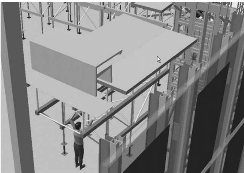
Fig. 14.10 One Island East: visualisation of working conditions (source: Baldwin et al. , 2008, Fig. 7.4).
