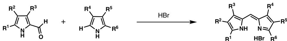
Figure 2. Synthesis of unsymmetric, 5-unsubstituted dipyrins by acid-catalyzed condensation reactions.
