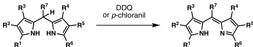
Figure 6. Synthesis of dipyrins by oxidation of dipyrromethanes.
