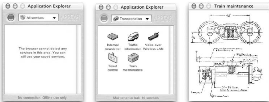
Figure 32.2: A typical end-user scenario where a maintenance worker automatically discovers available services on-site and can download and install interactive service manuals, etc. with a single click.
