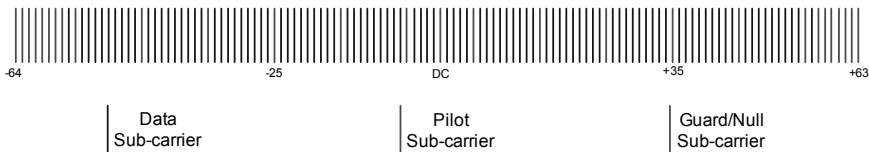
Figure 35.9: Sub-carrier allocation scheme for the WiMedia 1.0 PHY. Horizontal axis represents logical frequency bins.
