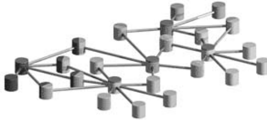
Figure 30.1: Concept of a small wireless sensor network, with wireless links shown as lines and embedded sensor nodes as cylinders.
