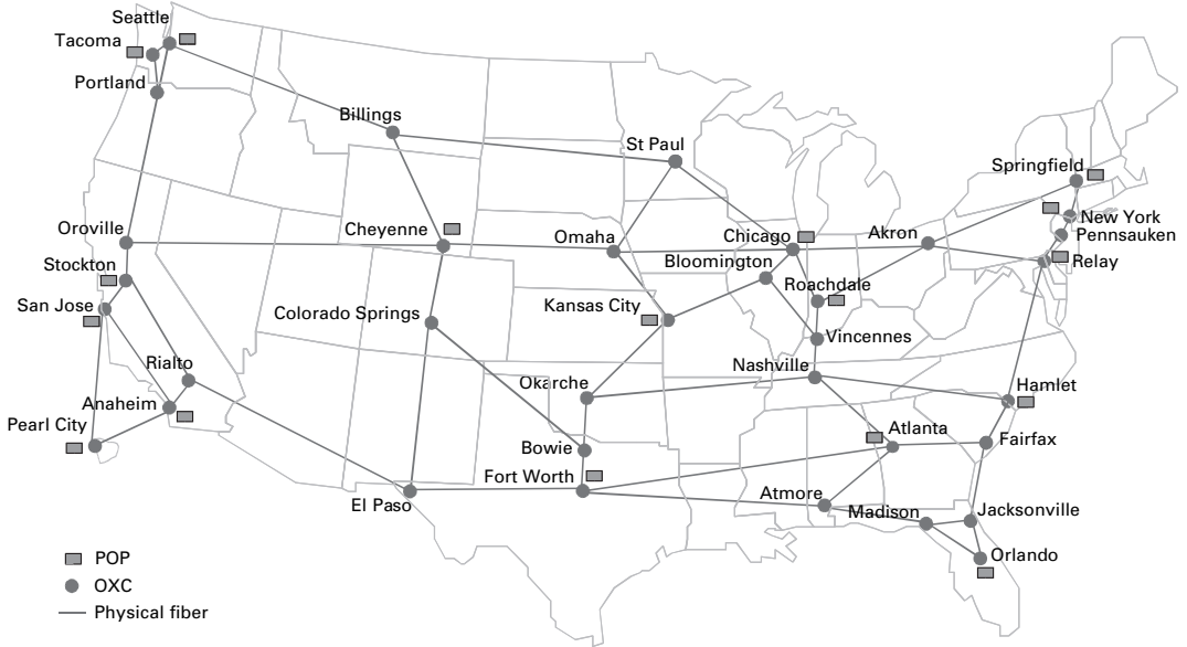
Fig. 2.4. North American Sprint fiber-optic backbone topology (third quarter, 2001, simplified version): 51 OXC and 77 WDM fibers.
