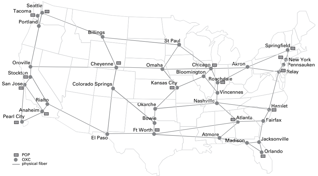
Fig. 8.4. North American Sprint fiber-optic backbone topology (third quarter, 2001, simplified version): 51 OXCs and 77 WDM fibers.
