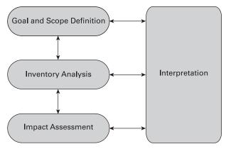
**Figure 9.2** The four iterative phases of a life cycle analysis (LCA) study according to ISO 14044
