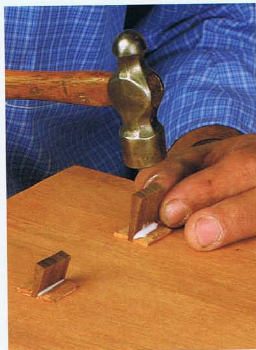
WALNUT WEDGES ADD CONTRAST. Cut the wedges to a 10° angle and tap them into the kerfs in the tenons until the tenons spread to fill the mortises.
