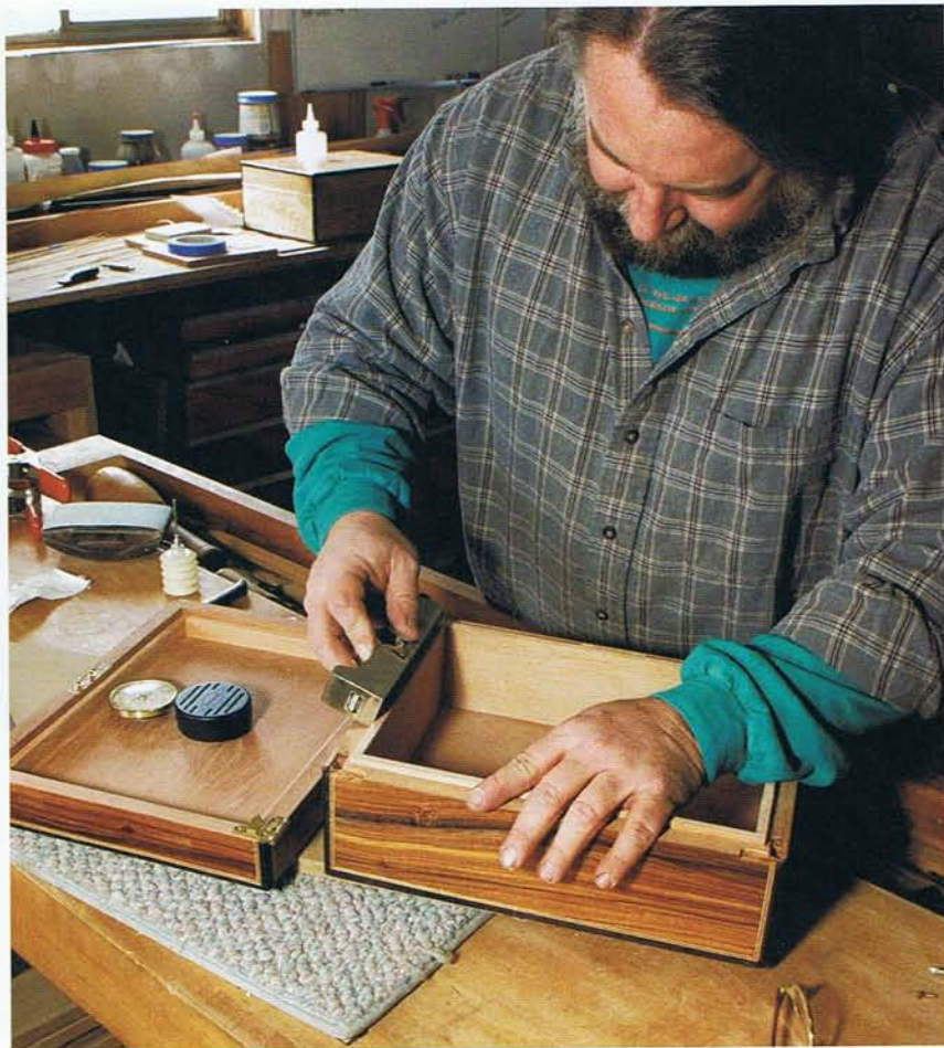
CAREFUL WITH THAT BEVEL ANGLE. It determines the rate the humidor loses humidity and receives fresh air. A humidor that is opened frequently should have a tighter fitting lid.
