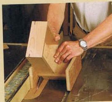
CUTTING KEYS. The carriage jig registers against the fence of the tablesaw and slides on two sleds.
