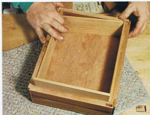
GENTLY PRESS-FIT THE LINING AROUND THE INTERIOR. When you season the humidor, the lining will swell and lock itself in place.
