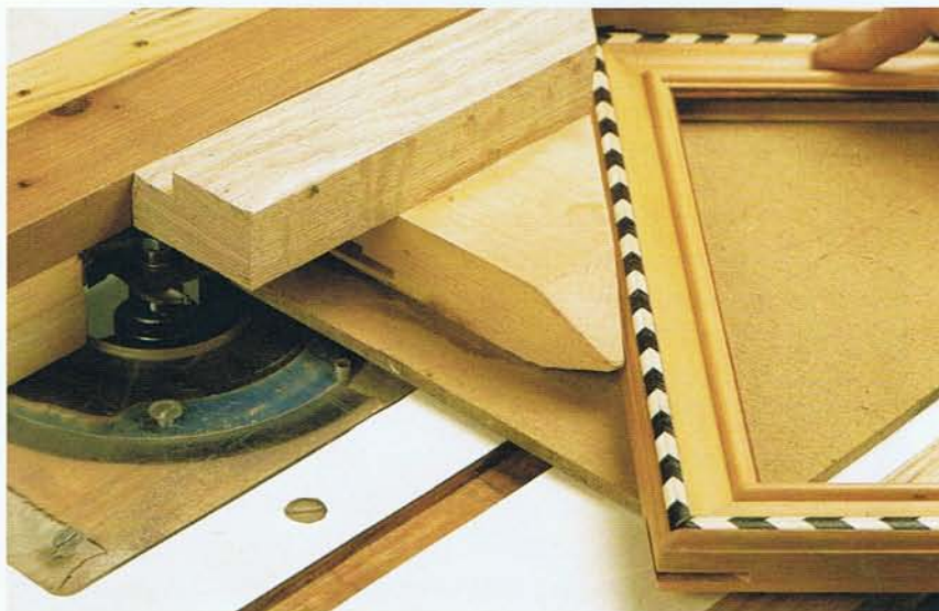
WITH A GROOVE-CUTTING JIG AND A SLOT-CUTTER in his router table, Segal plows grooves in this inlaid frame for the miter splines. The jig cradles the frame corner securely at a 45° angle to the fence and keeps his hands out of harm's way.
