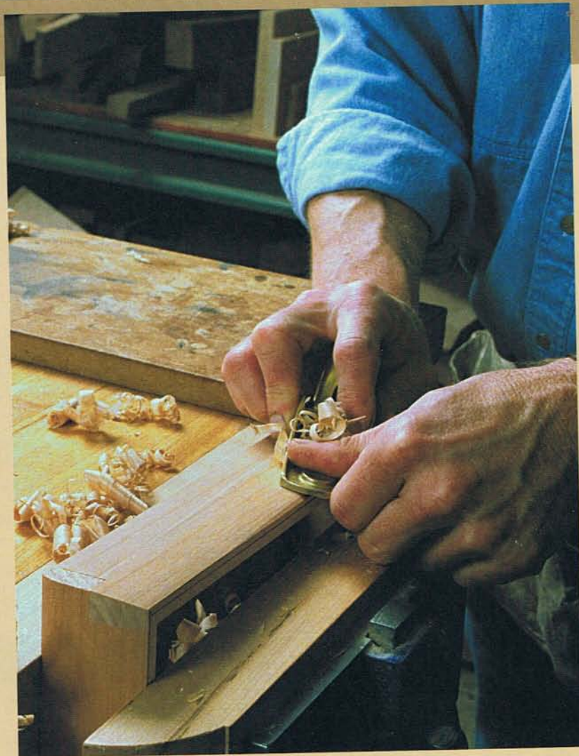
SHAPING THE TOP. The author uses a bench hook and a block plane (above) to round the top to a fair curve.
