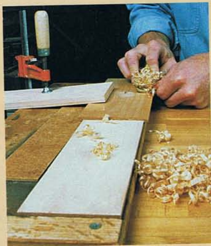
SHAPING THE TOP. The author uses a bench hook and a block plane (above) to round the top to a fair curve.
