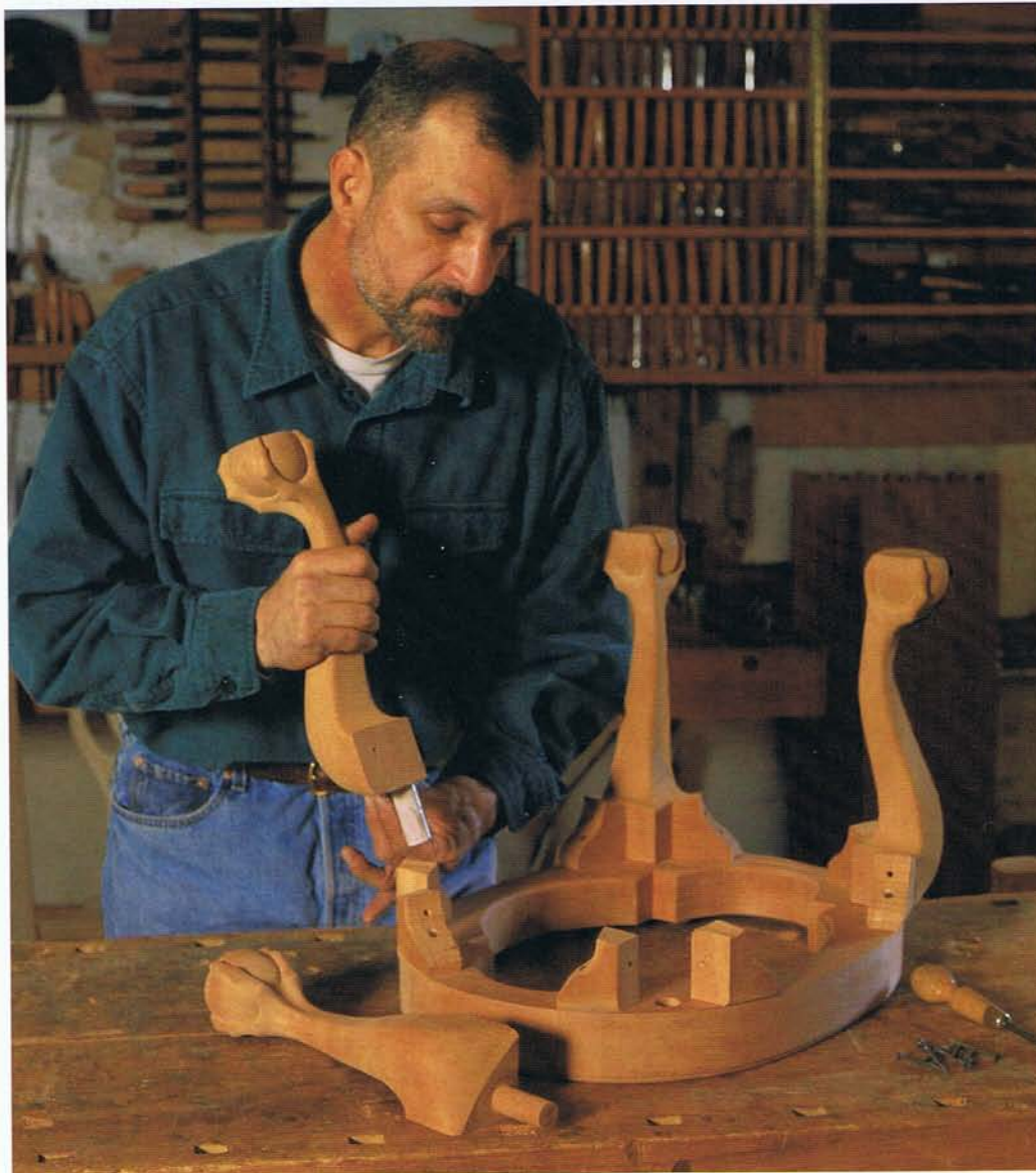
GLUE THE LEGS IN THE FRAME. The knee blocks temporarily screwed to the frame ensure that the legs go back in the same position. The knee blocks are glued in place after the leg glue joint has started to set.
