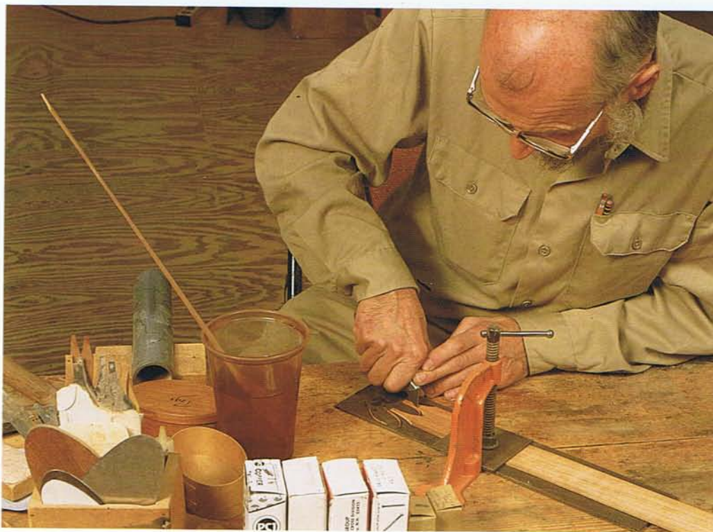
BEVELING THE FINGER EDGES AND ENDS is much easier if the band is first soaked in hot water and securely clamped to the bench. Reposition the hardboard cutting block for each finger set so that knife kerfs from previous cuts don't affect the cut.
