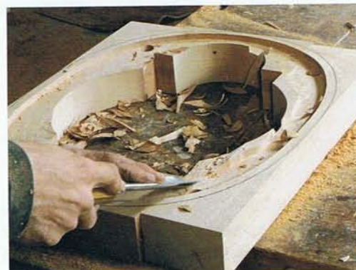
THIS GOUGE IS GOOD. To hog away stock the router couldn't reach, the author used a gouge.
