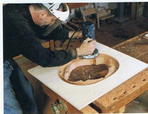
A ROUTER MAKES FAST WORK OF THE SEAT RABBET. Use a full-sized oval pattern to establish the layout line.
