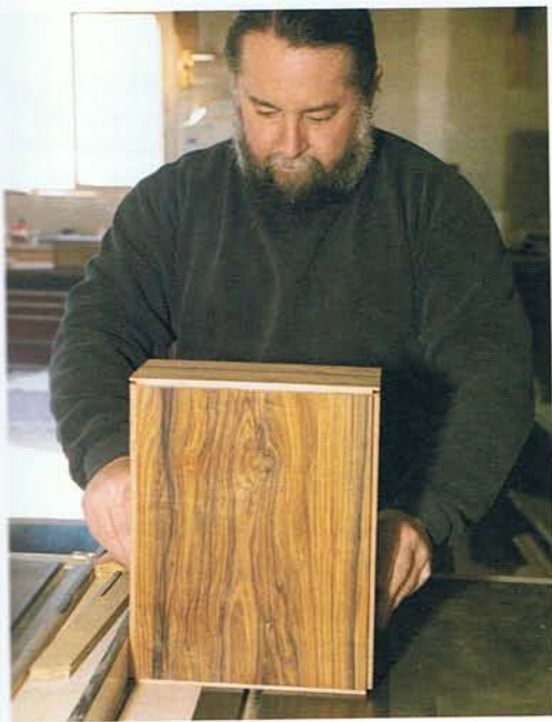
A TABLESAW MAKES THE EDGE-BANDING AND INLAY JOINTS A CINCH. Four cuts along each edge create the necessary joints.
