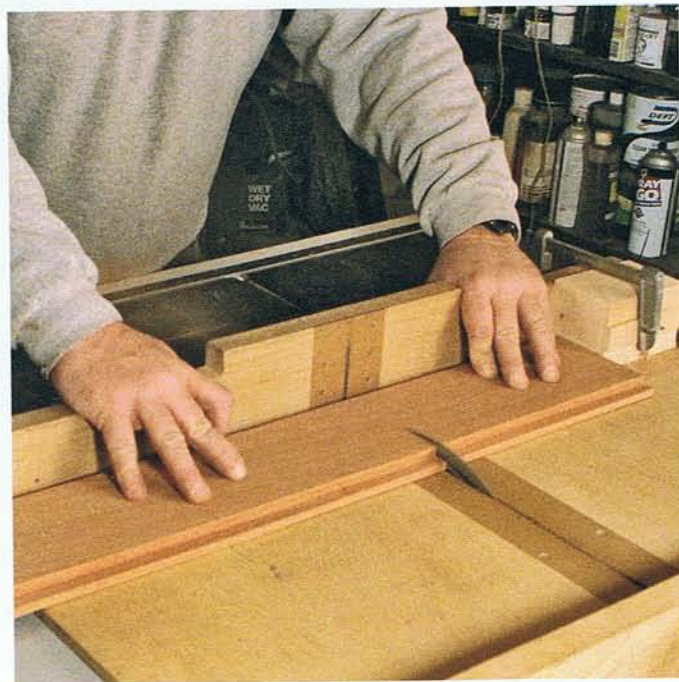
CUT THE RABBETED SIDES APART and to length on the tablesaw. Use a stop block to ensure consistent lengths.
