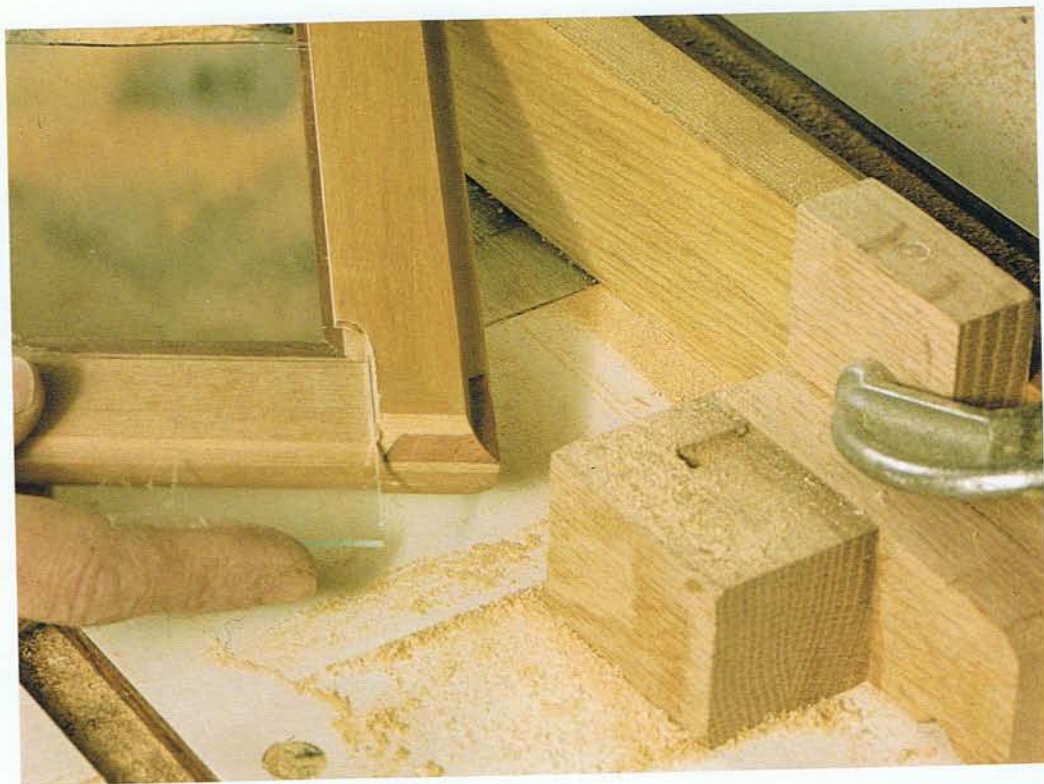
ACCESS SLOT. After routing a picture-entry slot by sliding this frame between two stop blocks on his router table, Segal checks the fit of the glass. The frame back was covered to show more of the spline.
