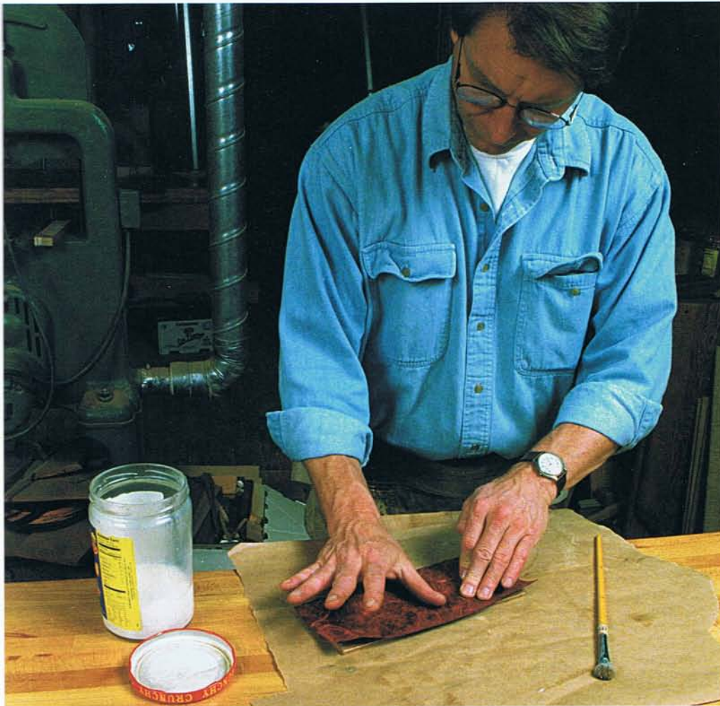
POLYURETHANE FINISH ACTS AS GLUE. The author brushes a coat of polyurethane onto a sheet of rice paper and the box bottom, then lays the paper on the bottom and lets it dry.
