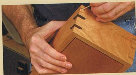
PREPARATIONS MAKE PERFECT. After a dry run with the band clamps set to the right length, apply glue to each mitered surface and assemble the box.
