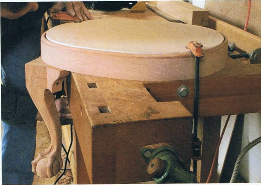
TEMPORARY FIXING. With the ball and claw complete, prepare to carve the knee by dry-fitting the leg to the frame. Use screws through the knee blocks to hold the leg in place.
