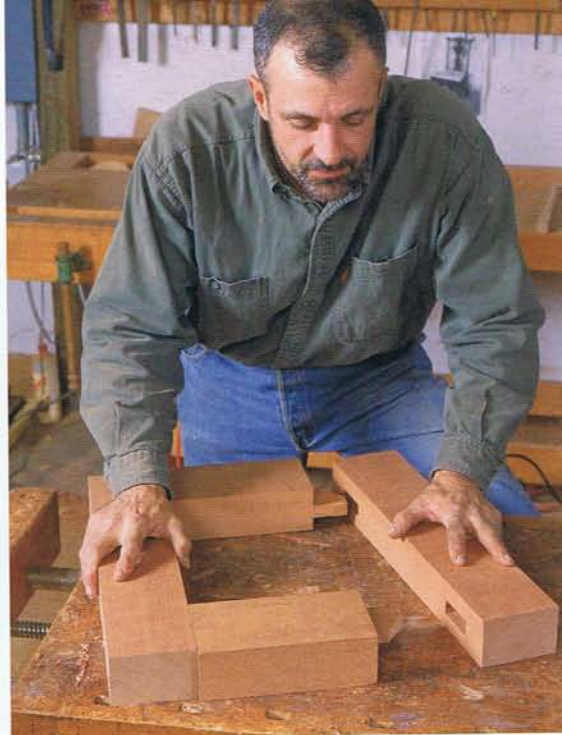
ASSEMBLE THE FRAME. The bulk of the frame has been reduced by bandsawing arc-shaped segments prior to assembly.
