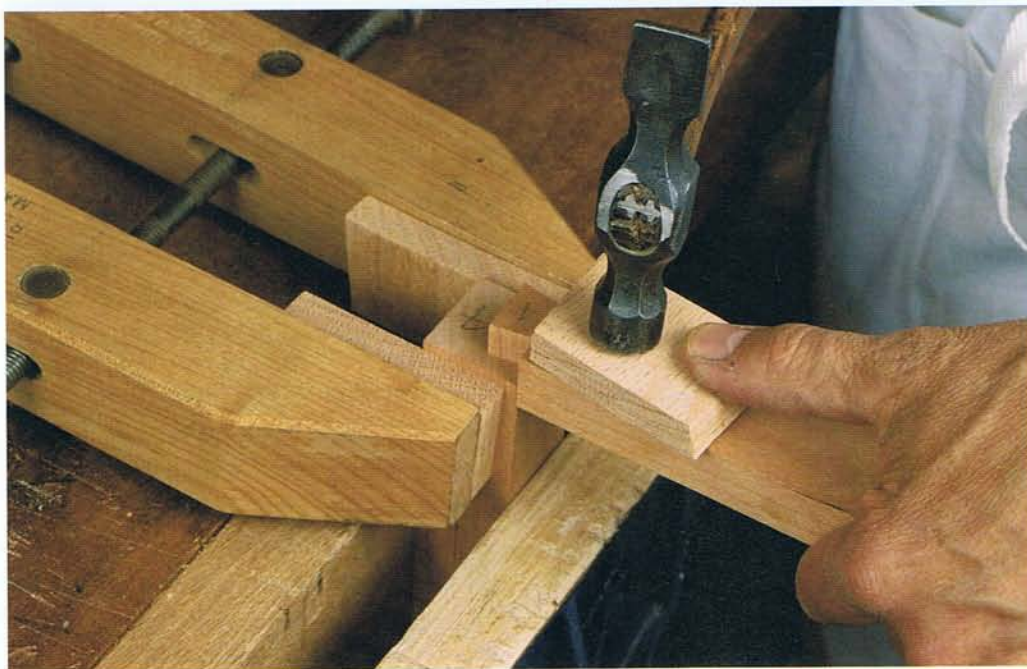
CHECKING THE FIT OF THE TOP-RAIL DOVETAIL. A handscrew prevents a leg from splitting if the dovetail is too big. The fit should be snug but not tight.
