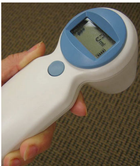
Fig. 8.21 An example of an automated bladder scanner. The automated bladder scan is useful for obtaining a post-void residual but is not considered a diagnostic ultrasound study
