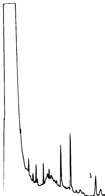
FIGURE 4-8. SFC chromatogram of a whole-blood extract of a bone marrow transplant patient with about 228 µg/l of CsA at 18.4 min. Pressure programming from 100 to 300 atm at 10 atm/min. Peak identification: 1, CsA. (From Wong, S. H. Y., et al., J. Liq. Chromatogr. Clin. Anal. , 17, 2093–2109, 1994. With permission.)
