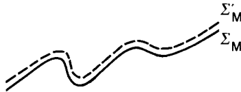
FIG. 1. Translation of the conductor equipotential surface in a displacement measurement.
