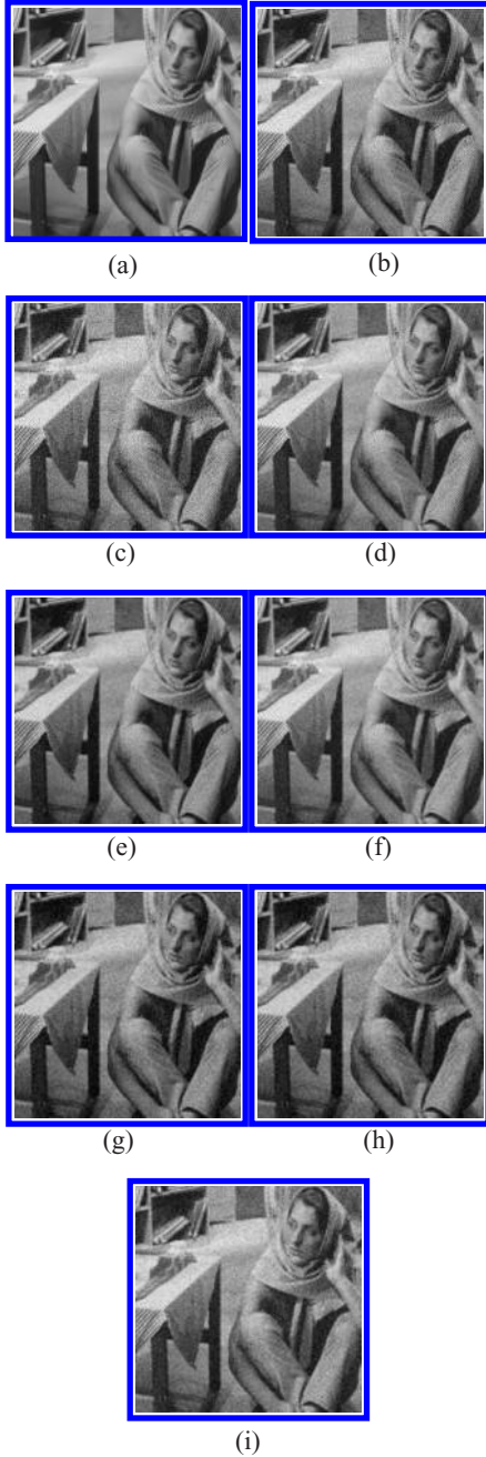
Figure 1. Denoising results of Barbara image. (a) The initial image; (b) The noisy image ( \sigma = 0.01 ); (c) The noisy image ( \sigma = 0.02 ); (d) Denoising results of WT to Figure 1b; (e) Denoising results of CT to Figure 1b; (f) Denoising results of CTPDE to Figure 1b; (g) Denoising results of WT to Figure 1c; (h) Denoising results of CT to Figure 1c; (i) Denoising results of CTPDE to Figure 1c.
