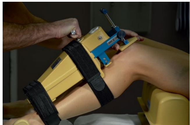
Fig. 5.6 This photo demonstrates the KT-1000 device positioned to measure posterior tibial translation
