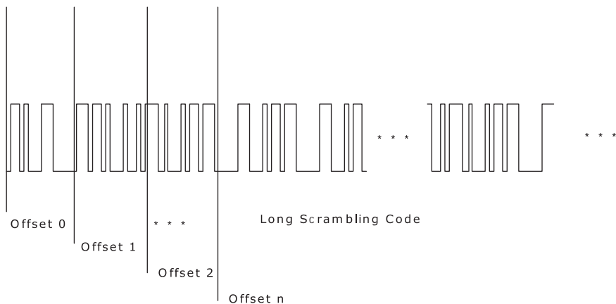
Figure 15.11 WCDMA scrambling codes with different offsets.
