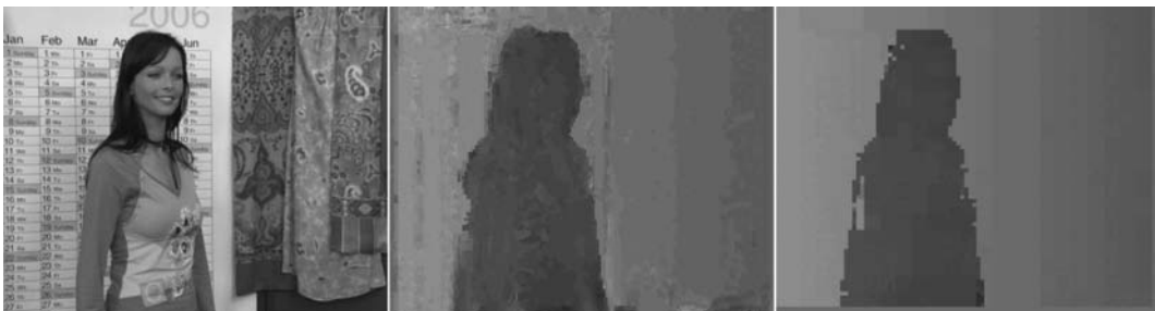
FIGURE 16.6 The horizontal component of the motion field estimated with the hierarchical logarithmic search (middle) and phase plane correlation (right) for the Yvonne sequence.
