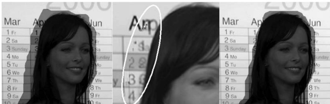
FIGURE 16.42 The extension of foreground motion vectors into background areas (left) leads to the so-called halo-artifact around moving foreground objects (middle). A motion estimator using three successive pictures leads to a more accurate vector field (right), but this is valid for the original image and not for the image to be interpolated.
