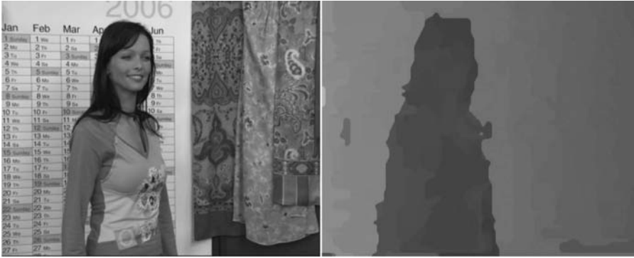
FIGURE 16.10 The horizontal component of the motion field estimated with 3DRS for the Yvonne sequence.
