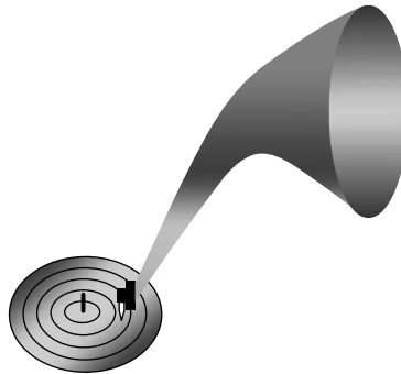
Figure 15.5 Illustration of the early acoustic recording process on a wax disc. Acoustic recordings were made by focusing the sound energy through a horn, via a sound box, diaphragm and stylus mechanism, onto a wax disc. The sound was distorted by reverberations of the horn.
