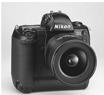
FIGURE 1.29 Mega-pixel digital still camera for newspaper photography (Nikon D1).
