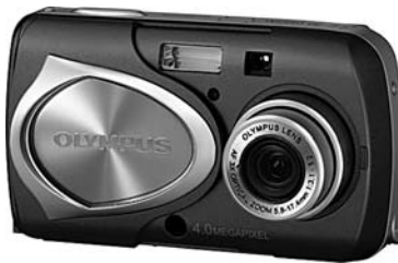
FIGURE 1.19 Point-and-shoot digital still camera with an optical finder.
