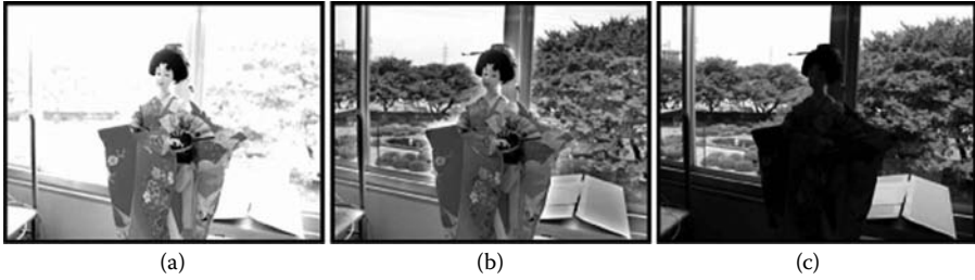
FIGURE 10.12 (See Color Figure 10.12 following page 178.) Example pictures: (a) with white clipping; (b) wide D-range; (c) with toneless black.
