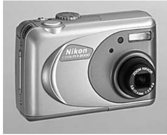
FIGURE 1.18 Point-and-shoot digital still camera with no optical finder.
