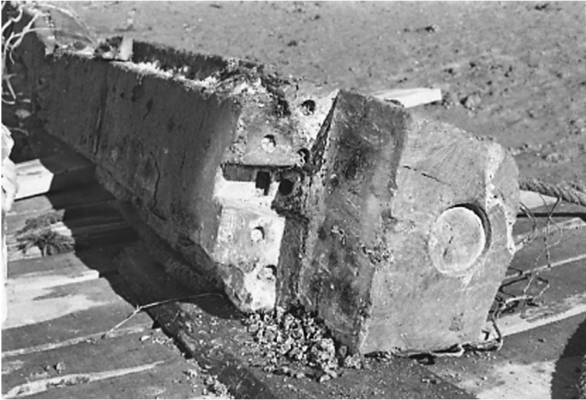
Figure 4.6. Scarf of the keel showing circular holes in which coins and a mirror could be placed. (Courtesy of Museum of Overseas Communication History)
