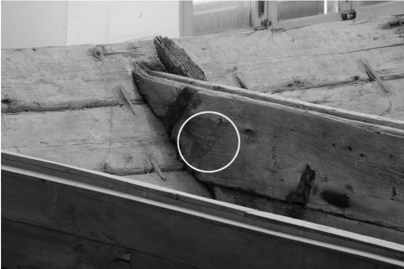
Figure 4.16. Part of a bulkhead plank ( inside the circle ) that shows evidence of recessing not completed. (Photo by author)
