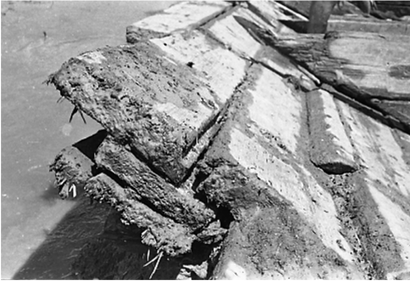
Figure 4.9. Three-layered hull planks showing rabbeted seams in the innermost planks. (Courtesy of Museum of Overseas Communication History)
