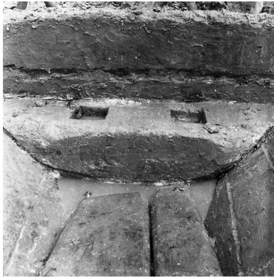
Figure 4.18. Photographs of the mainmast step ( above ) and forward mast step ( right ) after excavation. (Courtesy of Museum of Overseas Communication History)
