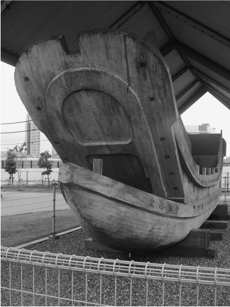
Figure 2.1. Reconstructed planked-up dugout canoe at the Osaka Maritime Museum; the lower part consists of a hollowed-out log. (Photo by author)
