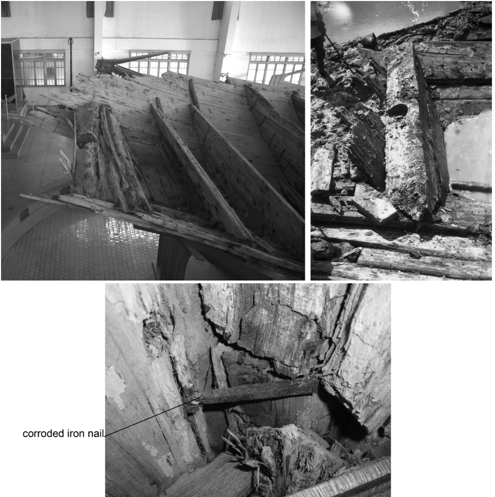
Figure 4.5. Stern of the Quanzhou ship at present ( top left ) and as recorded in a black and white photograph taken during the excavation ( top right ). Modern iron nail seen at the bottom of the hull ( bottom ). (New photos [top left and bottom] by author; older photo [top right], courtesy of Museum of Overseas Communication History)
