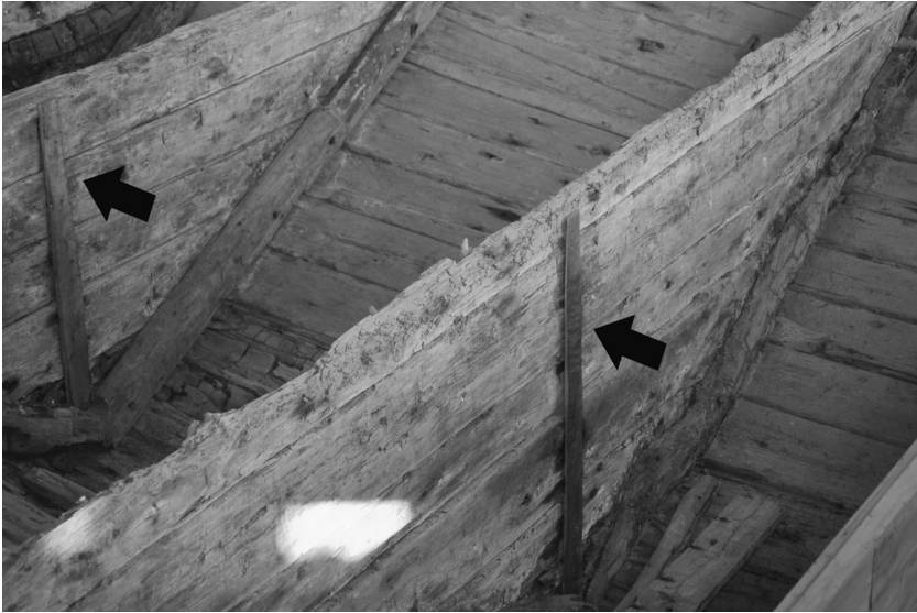
Figure 4.14. Vertical wooden strips in bulkheads nos. 10 and 11 represent the reconstruction of the original bulkhead stiffeners. (New photo [above] by author; older photo [left] courtesy of Museum of Overseas Communication History)
