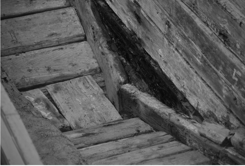
Figure 4.15. Bilge boards (or bottom ceiling planks) and the degraded bottom bulkhead plank. (New photo [above] by author; older photo [right] courtesy of Museum of Overseas Communication History)
