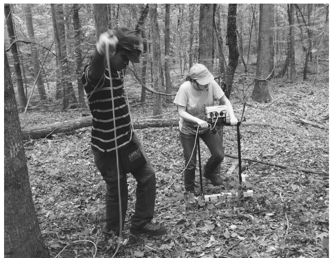
Figure 2. University of South Carolina anthropology students using a simple resistivity set at Williamston Farm Battlefield. Courtesy of the South Carolina Institute of Archaeology and Anthropology.
