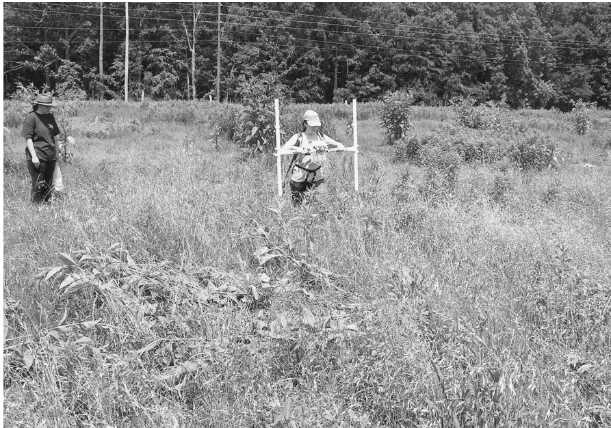
Figure 3. University of South Carolina anthropology students using a dual gradiometer rig at a historic farm site in Lower Richland. Courtesy of the South Carolina Institute of Archaeology and Anthropology.
