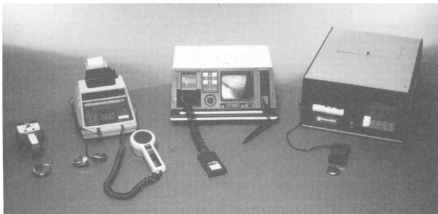
Figure 15.3 Pacemakers with their programmers. As pacemakers became smaller and more sophisticated their programmers became large and complex (left to right)
