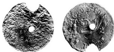
Figure 12.15. Aluminum token from Keeler, California, recovered from highly alkaline soil next to Owens Lake.
