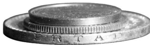
Figure G.6. Reeded edge displayed between a smooth edge and a lettered edge.
