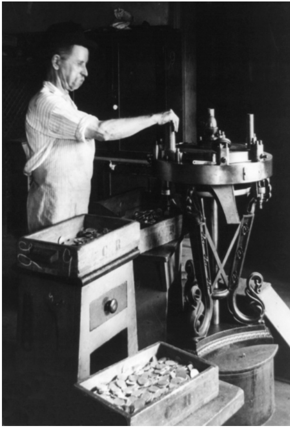
Figure 7.7. Milling blanks into flans, New Orleans mint, 1897. Photo by E. S. Gardner, 1897.
