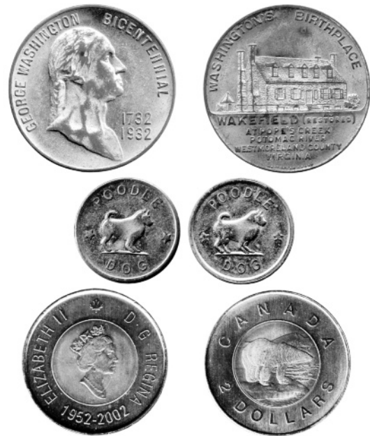
Figure 12.3. Metal plating. Gold-plated medal for the George Washington bicentennial in 1932, with plating worn off on the high points of the bust, revealing the copper beneath. Nickel plating on the pinball token of St. Paul, Minnesota's Poodle Dog Bar tended to wear off from the high points of the dog, showing the darker copper. Two distinctly different metals form the 2002 two-dollar coin of Canada.
