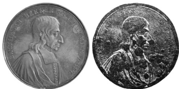
Figure 12.16. Tin pest was photographed in 1913 eating away at a Dutch, 1692, medal by Johannes Smeltzing honoring Reformed Church minister Balthasar Bekker, whose rationalist campaign against witch hunting cost him his pulpit. The photograph accompanied an article in Popular Science assessing the speed and destructiveness of tin pest. A medal in original condition is shown for comparison. Left image from the Amsterdam Museum.
