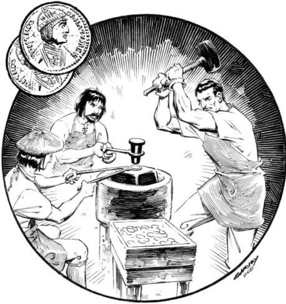
Figure 7.3. Striking coins between two dies with a hammer. Illustration by Brian Garvey.
