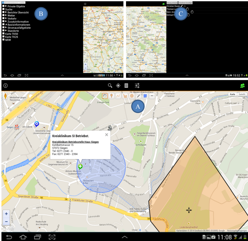
Figure 15: Screenshot of the mobile geo-collaboration system MoCo on tablet (A), the information pool to manage and select information resources (B) and the administration of the collaboration mode (C)
