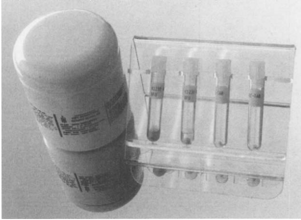
FIGURE 3 WEE-TABS stand-alone chromogenic tests. Each tube contains one tablet and a small volume of bacterial suspension.
