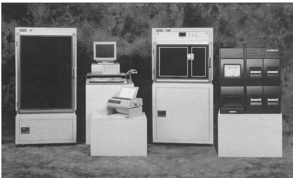
FIGURE 4 BacT/Alert system showing BacT/Alert 240 module (left), MB module (mycobacterial detection module) (right center), and 3D module (far right). Courtesy of Organon Teknika.
