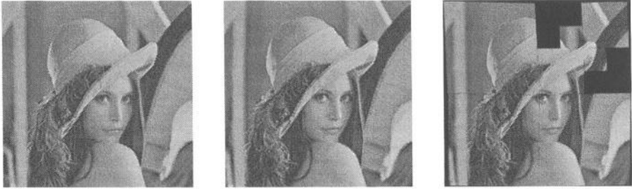
Fig. 7. An original watermarked image “lena.jpg” ( left ), an image attacked with Stirmark ( middle ), and a recovered image ( right ) – 64-bit watermark was decoded correctly
