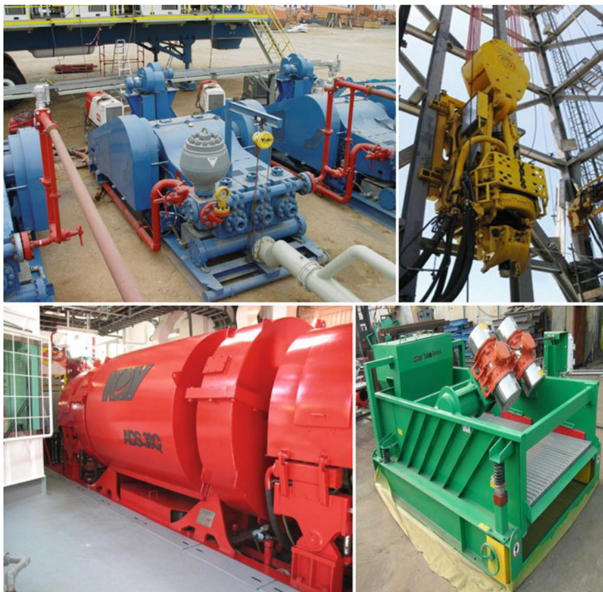
Fig. 15.2 Drilling equipment; Clockwise from upper left; mud pumps, top drive, shale shaker, drawworks
