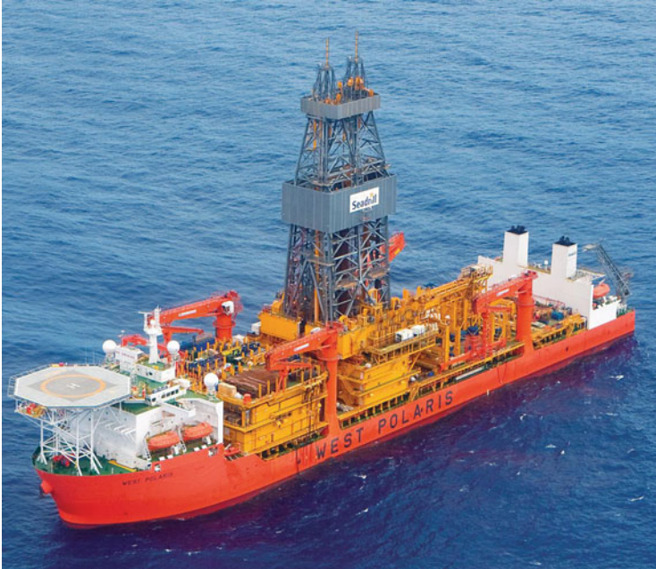
Fig. 1.20 Dual activity derrick on the sixth generation West Polaris drillship built in 2008 (Source: Seadrill)
