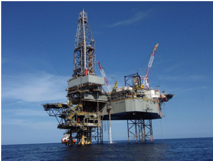
Fig. 1.12 A cantilevered jackup positioned over platform wells shown in the foreground (Source: Seadrill)
