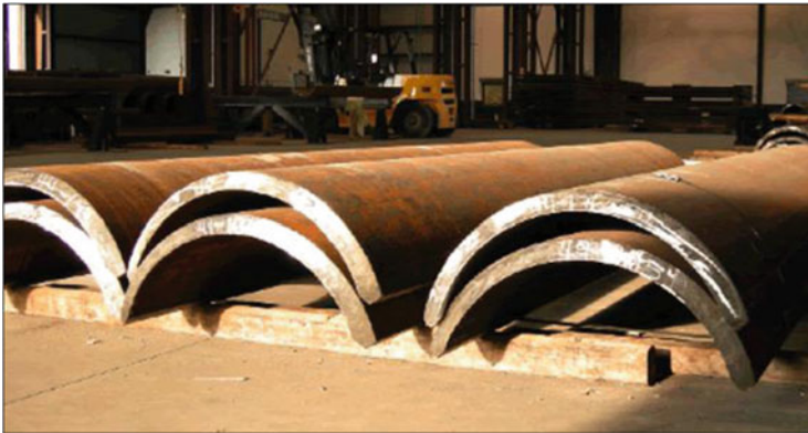
Fig. 11.7 Formed half chords (Source: Jackrabbit Steel)
