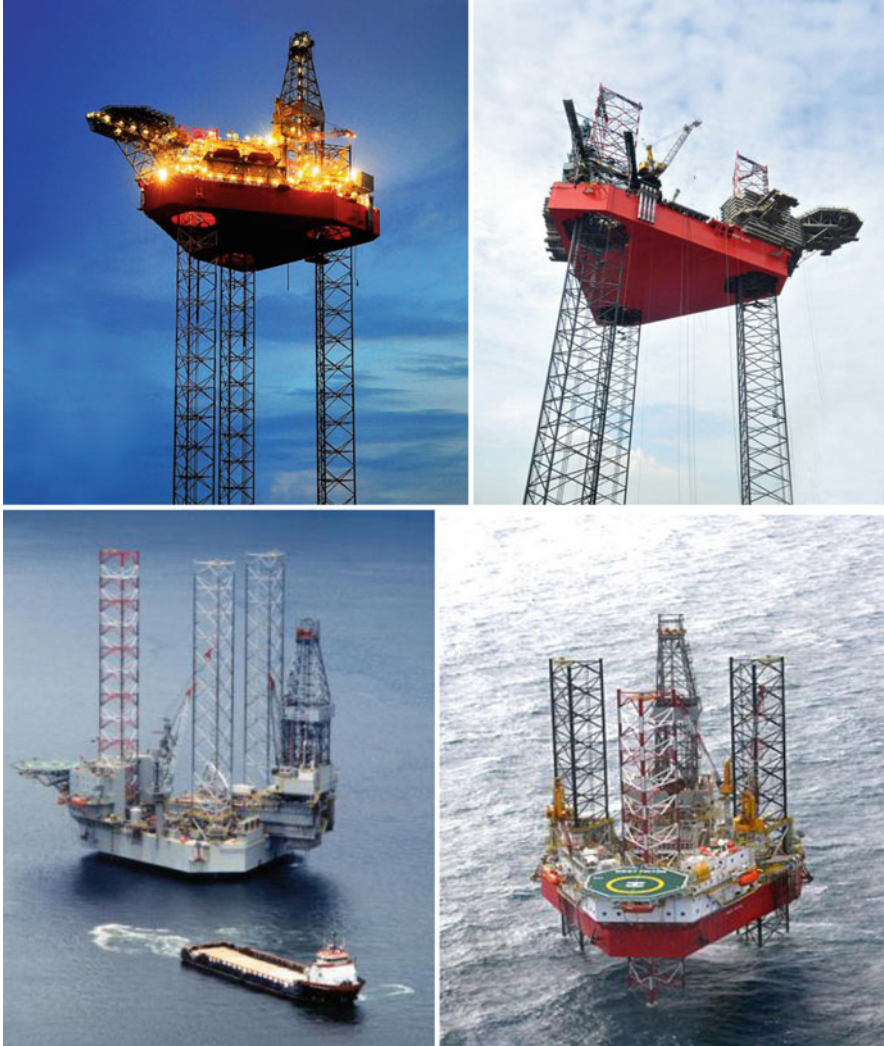
Fig. 10.16 Commonly built international jackups; clockwise from top left : KFELS B Class, Gusto MSC CJ70, Pacific Class 375, F&G JU 2000E (Sources: Seadrill; Freide and Goldman)
