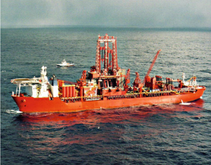
Fig. 1.19 A modern drillship, the fifth generation West Navigator built in 2000 (Source: Seadrill)
