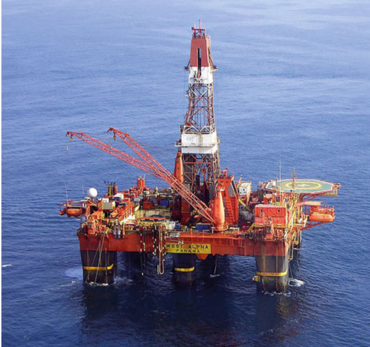
Fig. 1.15 The West Alpha , a fourth generation semisubmersible built in 1986 (Source: Seadrill)
