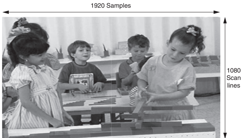
Figure 5.38: Scaling 4:3 content for a 16:9 display: “Panorama” mode. Left and right 25% edges of picture are nonlinearly scaled horizontally to fill 16:9 display, distorted picture on left and right sides
