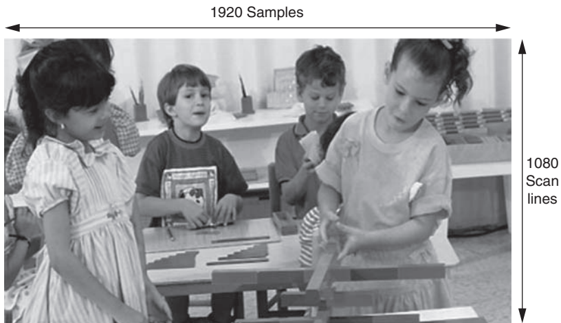
Figure 5.37: Scaling 4:3 content for a 16:9 display: “Zoom” mode. Top and bottom portion of 4:3 picture deleted, then scaled to fill 16:9 display
