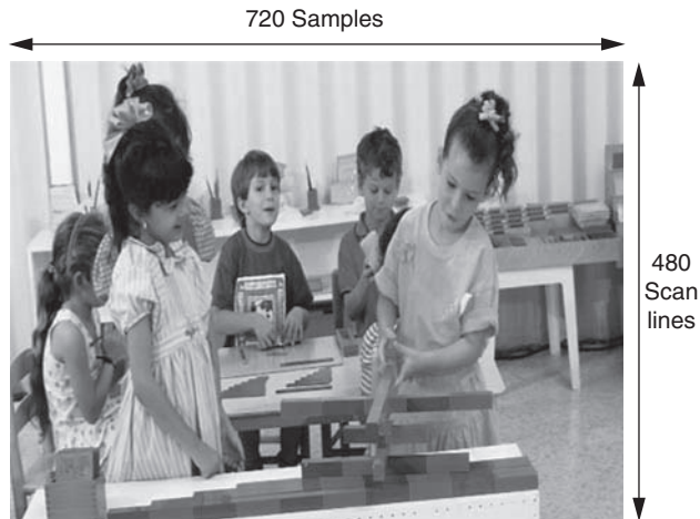
Figure 5.33: Scaling 16:9 content for a 4:3 display: “Squeezed” mode. Entire 16:9 program horizontally squeezed to fit 4:3 display, resulting in a distorted picture
