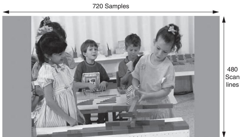
Figure 5.31: Scaling 16:9 content for a 4:3 display: “Normal” or pan-and-scan mode. Results in some of the 16:9 content being ignored (indicated by gray regions)
