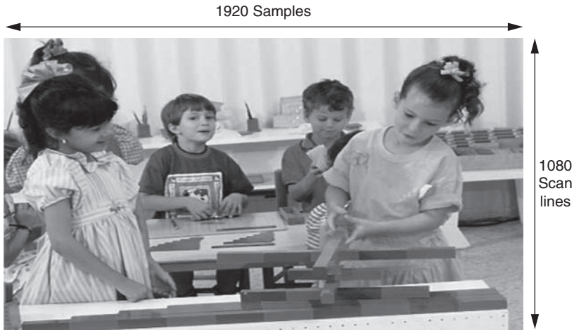
Figure 5.36: Scaling 4:3 content for a 16:9 display: “Wide” mode. Entire picture linearly scaled horizontally to fill 16:9 display, resulting in distorted picture unless used with anamorphic content
