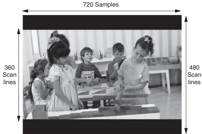
Figure 5.32: Scaling 16:9 content for a 4:3 display: “Letterbox” mode. Entire 16:9 program visible, with black bars at top and bottom of display
