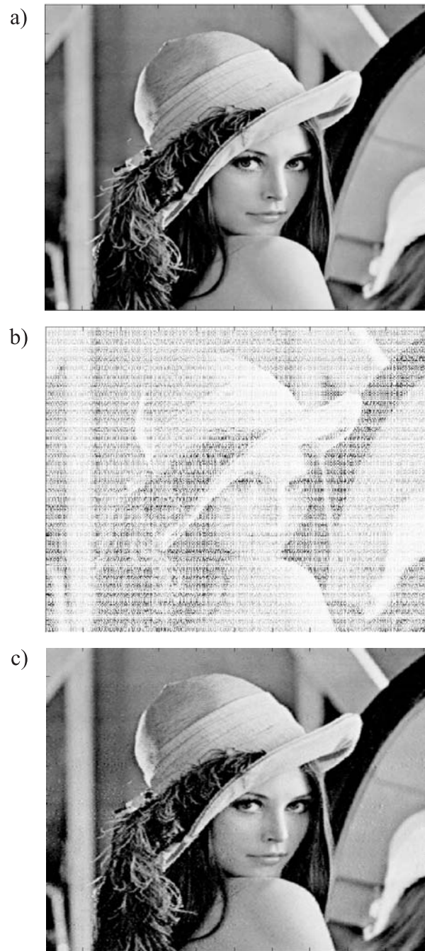
Figure 20.11 Illustration of two-dimensional data compressed four times and reconstruction of the respective image: (a) original image; (b) compressed image with 75 % of the pixels taken out; (c) reconstructed image
