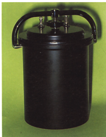
Figure 8.5 Anaerobic jars are airtight containers of metal or clear plastic within which an anaerobic atmosphere can be generated for the isolation of strict anaerobes
