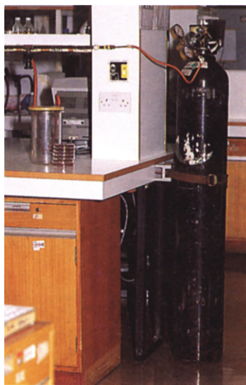
Figure 8.7 While plates are waiting to be placed in a cabinet or jar they can be placed in a holding jar which resembles an anaerobic jar but is connected to a CO 2 cylinder
