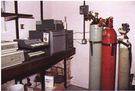
Figure 8.3 Gas-liquid chromatography. The three-fold gas supply leads to the chromatograph which contains a long column with specialized packing material and a flame ionizer. The pen recorder provides a written record of the tracing
