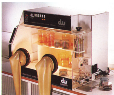
Figure 8.6 An alternative to the anaerobic jar is the anaerobic cabinet which permits the manipulation of cultures through the glove ports. Cultures and plates enter through the airlock at the side
