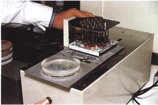
Figure 20.7 Multi-point inoculator is used to inoculate plates in the agar incorporation MIC method
