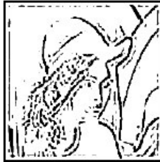
Figure 6.21 – Results of the thresholding after derivative filtering
