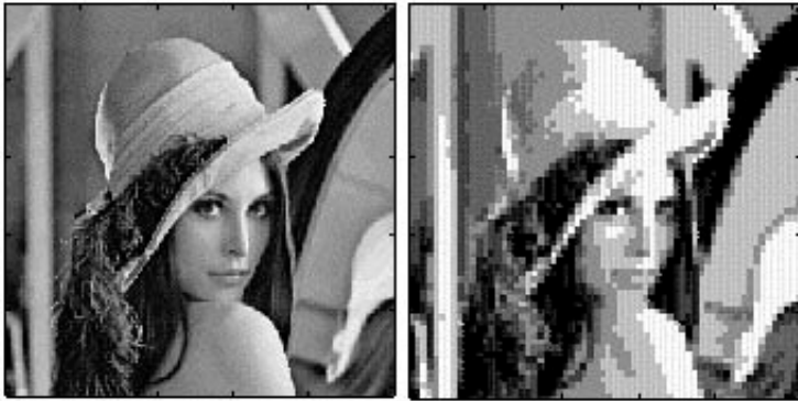
Figure 12.37 – Original image on the left and the result of the LBG compression with m = 16 and b = 3
