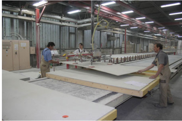
Fig. 3.33 Production of load-bearing wall elements in a factory
