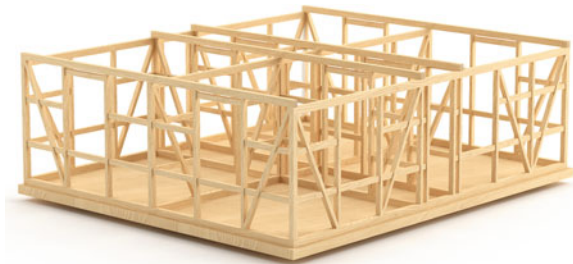
Fig. 3.27 First signs of prefabrication in timber-frame construction
