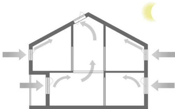
Fig. 2.23 Convective nighttime cooling by means of ventilation
