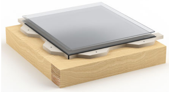
Fig. 4.28 Connection of the glazing to the substructure and the timber frame in HGV elements, adopted from Neubauer and Schober [44], Holzforschung Austria, Pat.-Nr. 502470
