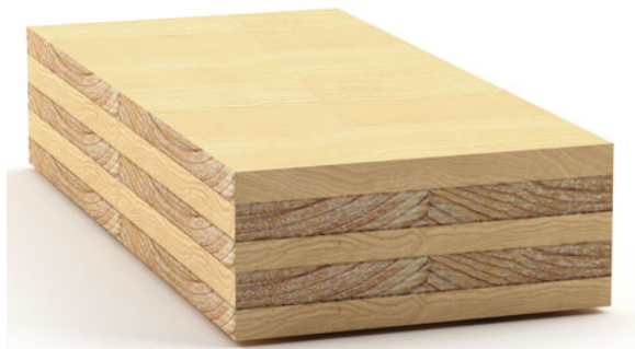
Fig. 3.20 LenoTec product with 5 spruce fir plies glued together crosswise, t = 135 mm, 5 plies
