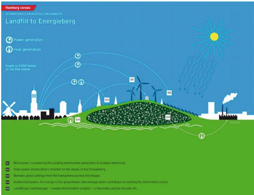
Fig. 5 Cross section of Wilhelmsburg Energie Colline Georgswerder (Source Energy Atlas IBA—Hamburg)
