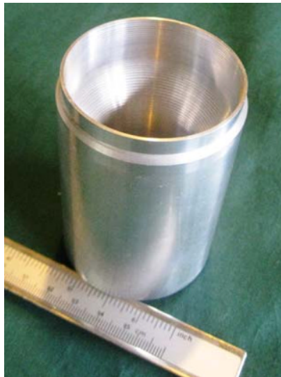
Figure 4.44 Smooth wall circular horn with aperture diameter 2\lambda designed for maximum gain and low cross-polarization
