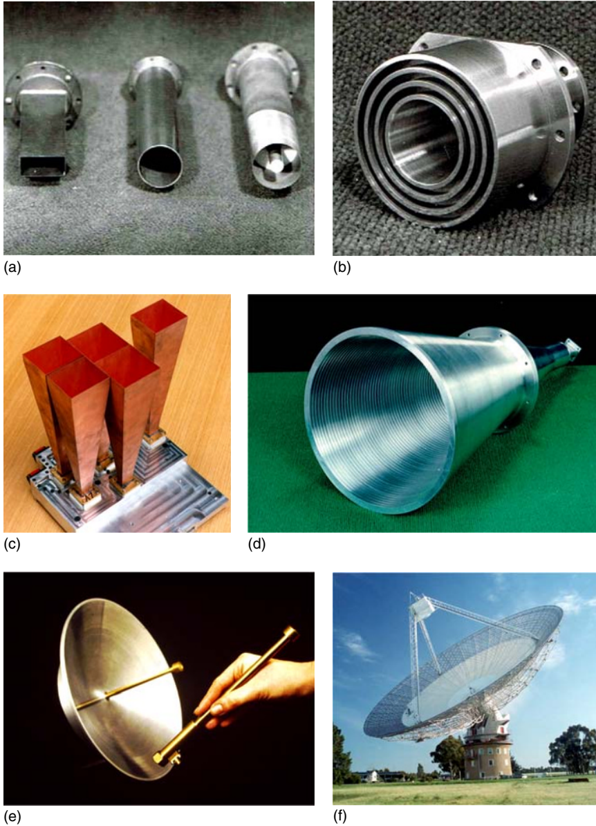
Figure 1.1 Examples of aperture antennas. (a) Open-ended waveguide antennas (right to left) coaxial, circular and rectangular. (b) Circular waveguide (diameter 32.7 mm) with three ring-slots designed for operation at 9 GHz. (c) Feed array of pyramidal horns for 12.25–12.75 GHz. (d) 11–14.5 GHz high-performance circular corrugated feed horn, diameter 273 mm, and flare angle 11.8^\circ . (e) Small paraboloidal reflector and rear waveguide feed designed for a 15 GHz microwave link. (f) 64 m Parkes radio telescope is a front-fed paraboloid ( f/D = 0.408 ). This versatile instrument has been used for frequencies from 30 MHz to >90 GHz. Source: Reproduced with permission from CSIRO (a–f)
