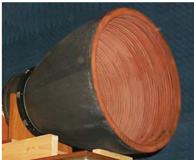
Figure 10.10 Low-sidelobe horn manufactured in carbon fibre and copper coated is its interior for high performance. Source: Reproduced with permission from CSIRO
