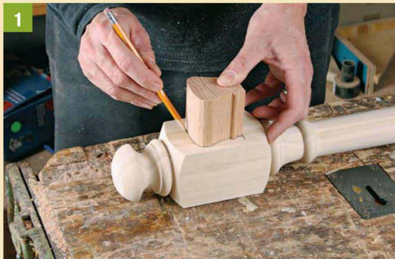
1 Trace the rail profile onto the newel.
