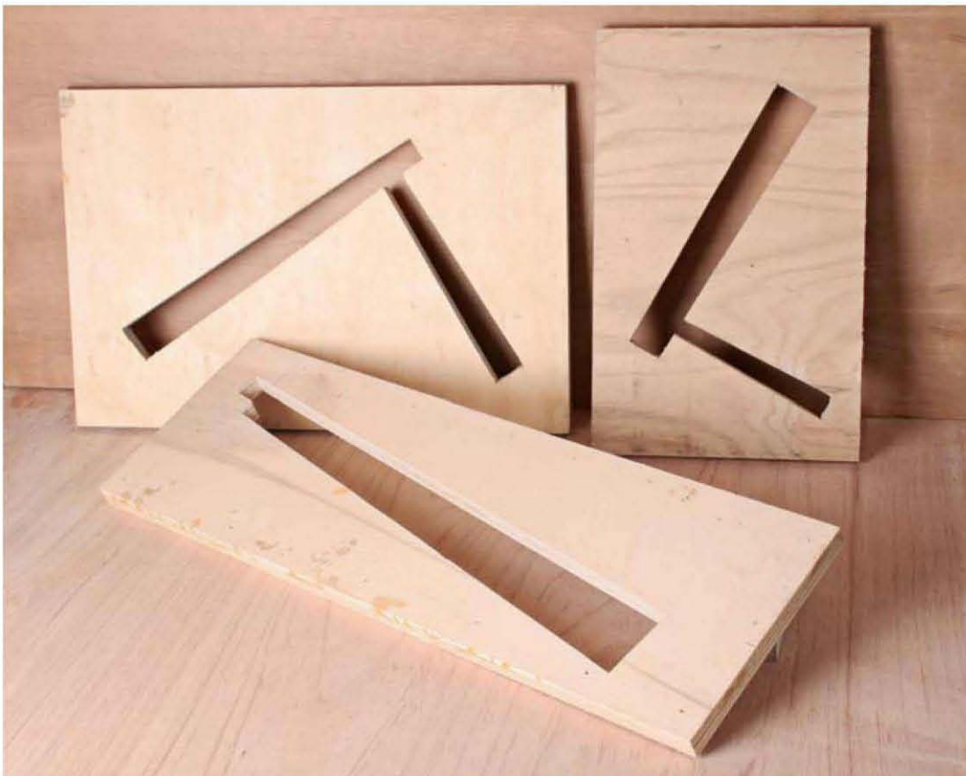
The lower, longest mortise jig is for routing wide treads in winder stairs. The one on the left is most typical, for use with 5/4 treads and 4/4 risers. The right hand jig is for 2x treads.
