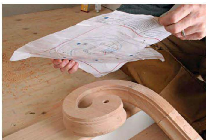
The volute template is finally used on the volute. Before assembling the volute and the quarter-turn with epoxy and a rail bolt, mark and drill the volute for balusters.
