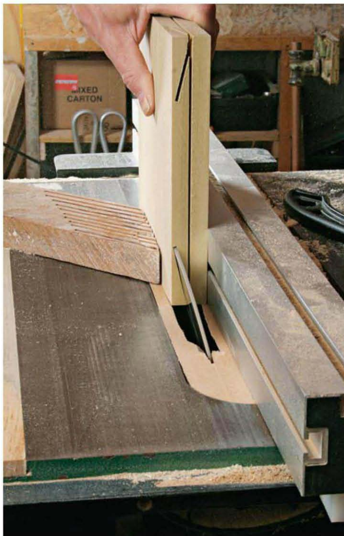
Bevel the cap with a tablesaw. This cap has a 2-in.-wide bevel of about 15°. The featherboard helps to prevent kickback and ensure consistent cuts.
