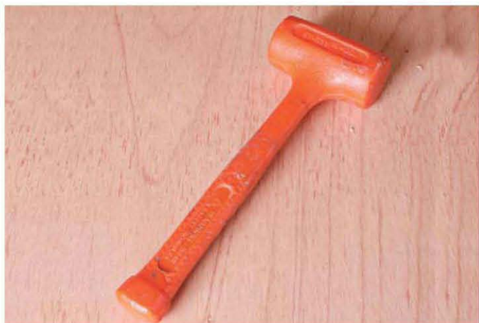
Dead-blow hammers don't leave dents. The color's a grabber too.
