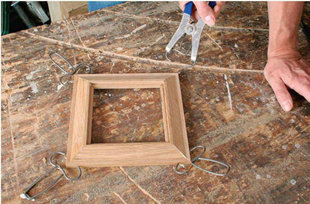
Spring clamps are inexpensive, leave holes smaller than a finish nail, and exert plenty of pressure to glue up the frame.
