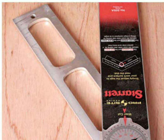
A Starrett protractor is a grand tool for measuring angles. It has two scales: one provides the measurement of the angle in degrees and the other displays the miter angle.
