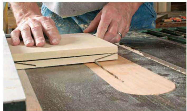
Shallow cuts finish the cap bevels. Be careful not to overcut—it's easier to pare off a little extra material than it is to repair a saw kerf into the bevel.
