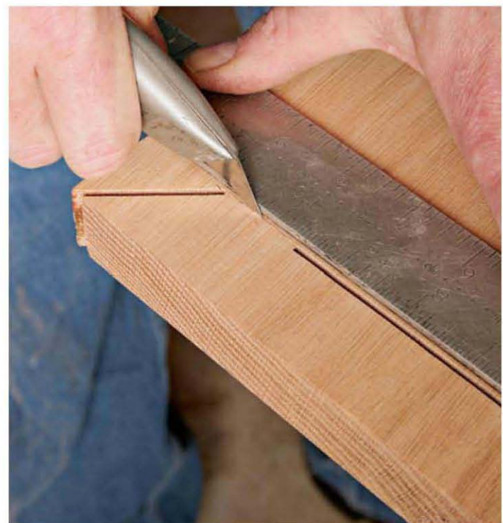
Splintering is easily avoided. Knife-cut the line of the return before sawing it to make a crisp edge.
