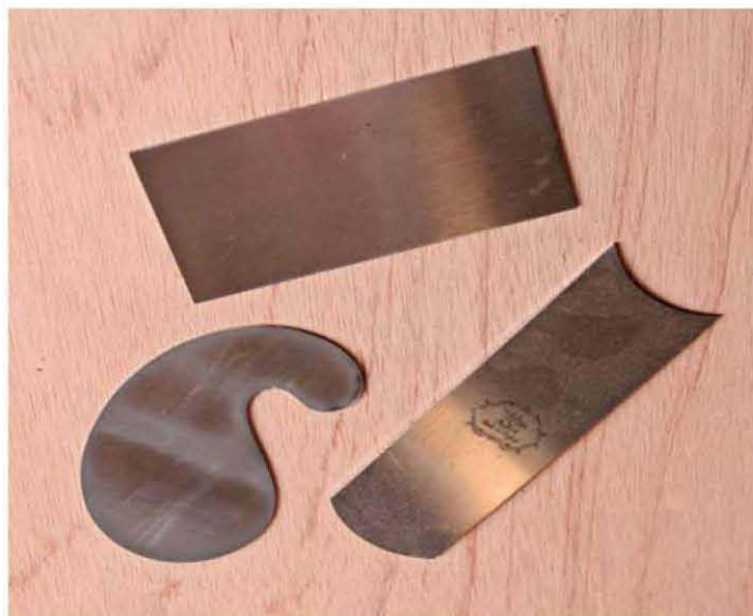
Cabinet scrapers are cheap, faster than hand sanding, and easy to resharpen.
