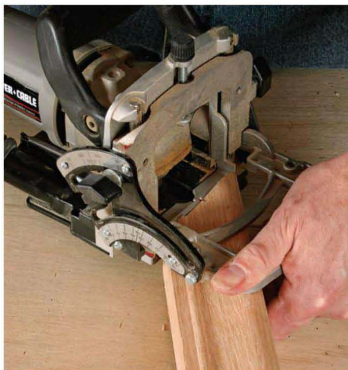
Biscuits join the halves of the railing drop. After holding the halves together and marking the center of the joint, cut a #20 slot from each side of the rail with the biscuit joiner resting on its high and low points.
