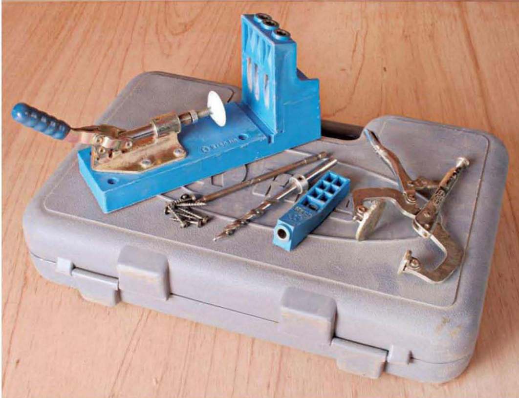
Pocket hole jigs guide a special bit to create an oblique pilot hole.
