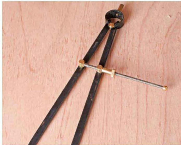
Twelve-inch dividers (Lee Valley Tools, Ltd., 1-800-267-8735, www.leevalley.com ) are indispensable for laying out winder stairs.
