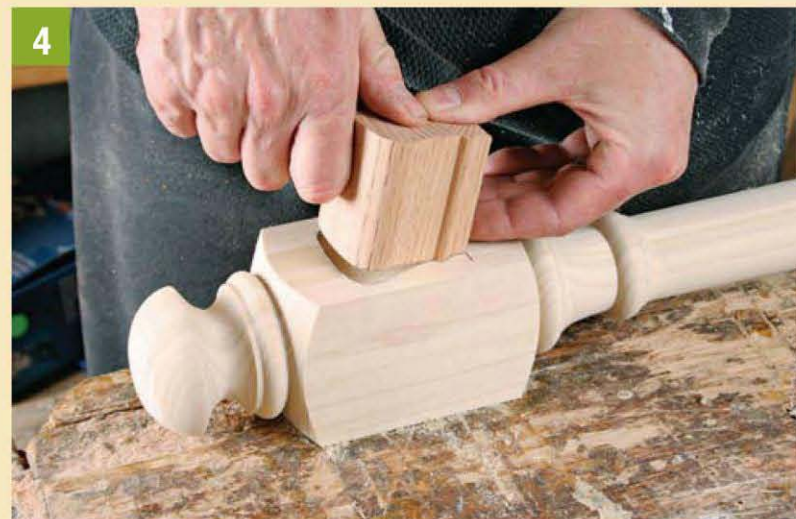
4 Test-fit the rail.
