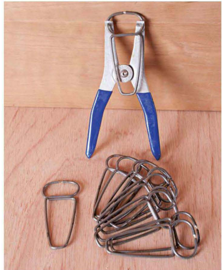
Spring miter clamps leave holes smaller than most finish nails.
