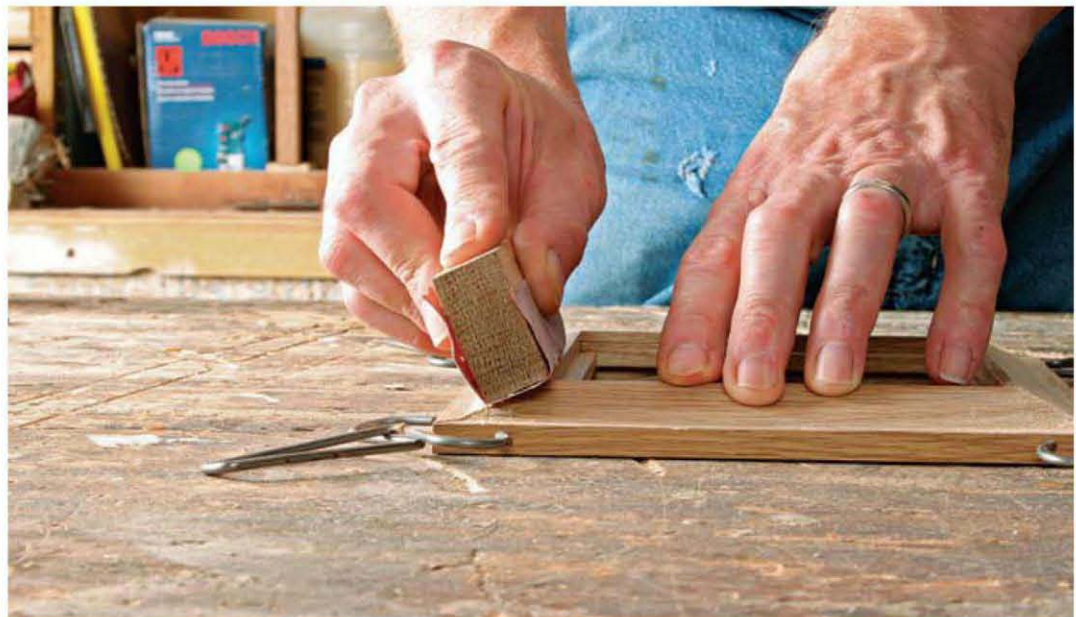
Sanding down the high side levels an imperfectly matched joint, making it look as if it were perfectly cut and assembled.
