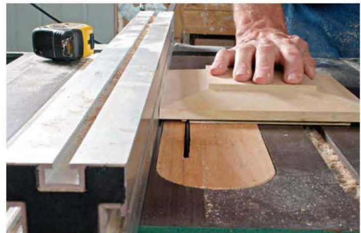
Recess the bottom of the cap. Remove enough material to create a square knob on the cap's bottom that will seat in the chair-rail cap.
