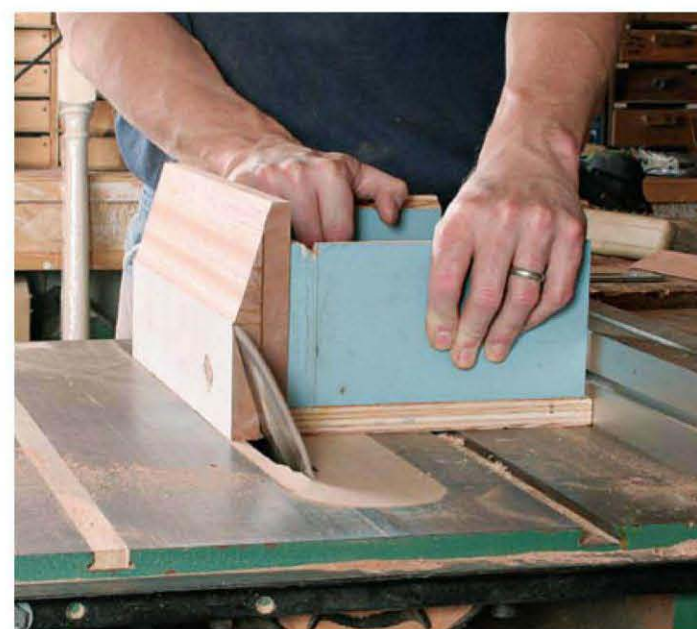
Bevel the caps using a sled. Screwed from the inside to a plywood box sled, the stock for the cap receives its second bevel.
