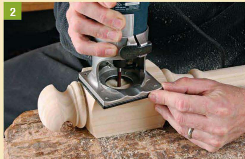
2 Carefully rout to the line.
