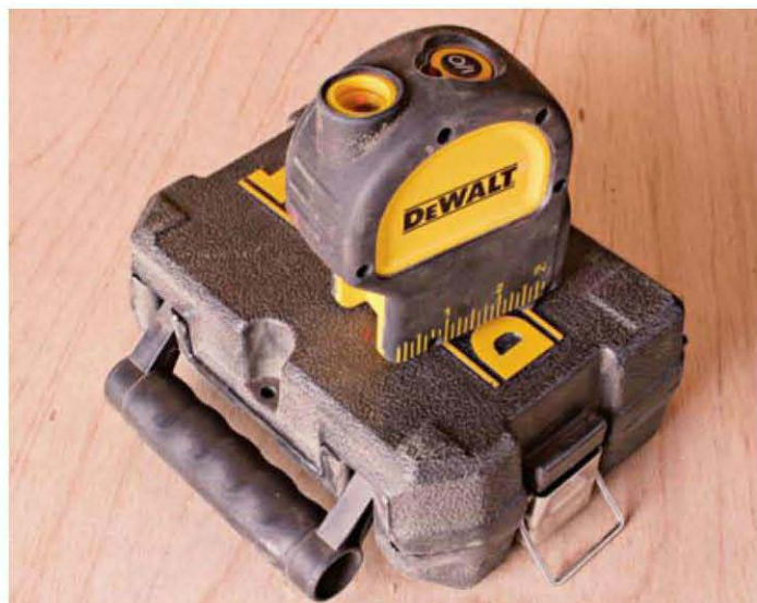
A laser plumb bob speeds initial layout and could be used to transfer the location of balusters from the treads to the railing (DeWalt, 800-433-9258, www.dewalt.com ).
