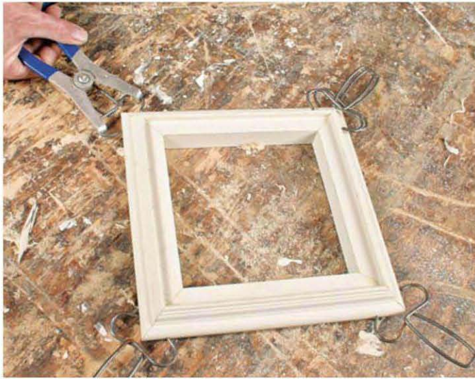
A frame of stock chair-rail cap tops the newel. Other rabbeted moldings, such as window stool, could also be used here.
