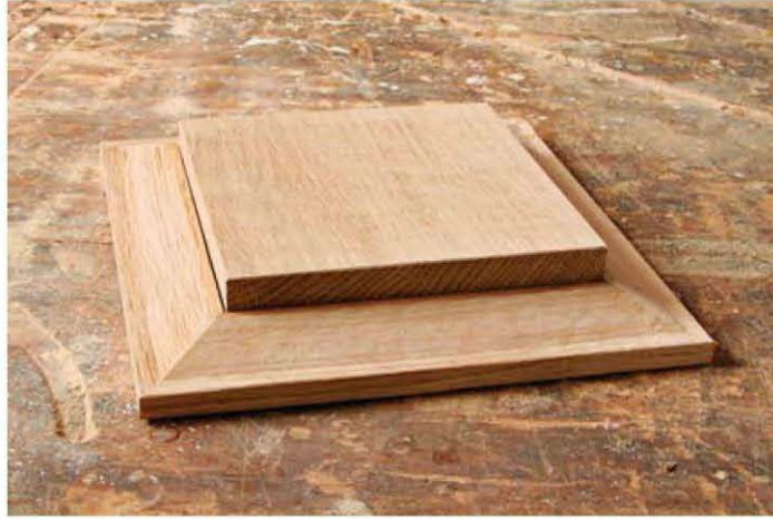
Built-up caps are composed of molded stock put together like a picture frame and a top block that sits inside the frame.
