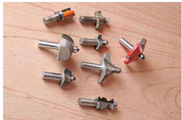
The bits used to produce a variety of molded shapes all have ½-in. shanks. Except for the lightest work, ¼-in. shanks aren't acceptable.
