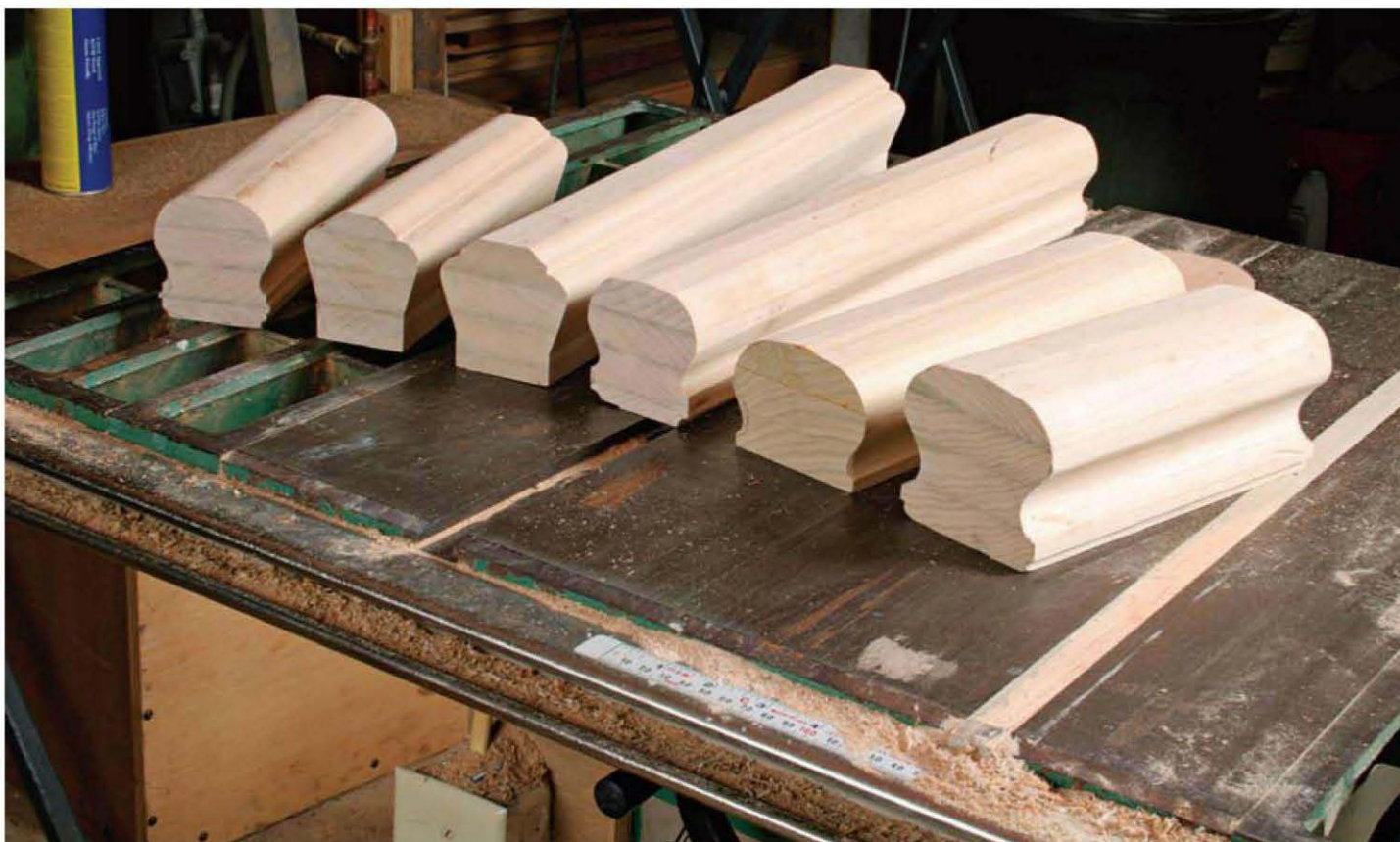
These railing samples were all made using a tablesaw and a router table fitted with stock railing bits available from any good supplier.
