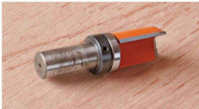
The bits used to produce a variety of molded shapes all have ½-in. shanks. Except for the lightest work, ¼-in. shanks aren't acceptable.
