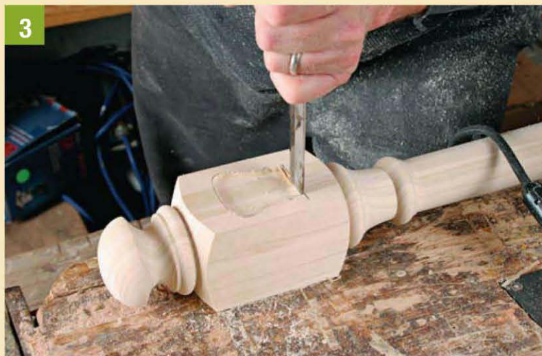
3 Square the corners with a paring chisel.
