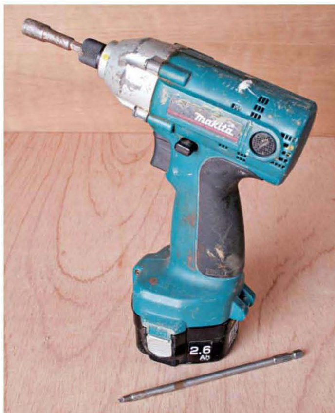
Impact drivers are used to drive screws when the going gets tough.
