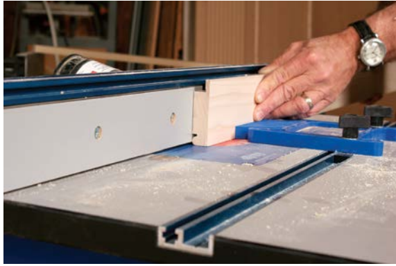
AFTER THE DOOR-FRAME STOCK IS CUT TO WIDTH and rabbeted to receive the panel, rout the other edge with a \frac{3}{8} -in. beading bit.
