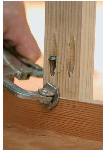
SQUEEZE THE GRAIN TO ELIMINATE SPLITTING. Put a bit of wood glue on the board end before securing a locking C-clamp so that it exerts equal pressure on the grain of each component. The clamp should be placed in line with the pocket hole being screwed.
