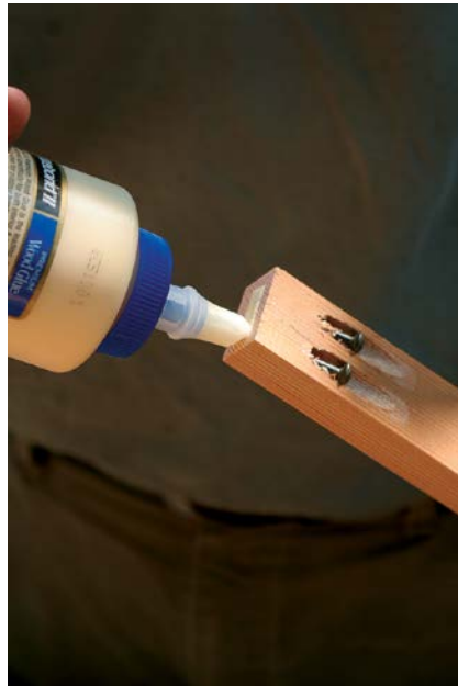
SQUEEZE THE GRAIN TO ELIMINATE SPLITTING. Put a bit of wood glue on the board end before securing a locking C-clamp so that it exerts equal pressure on the grain of each component. The clamp should be placed in line with the pocket hole being screwed.
