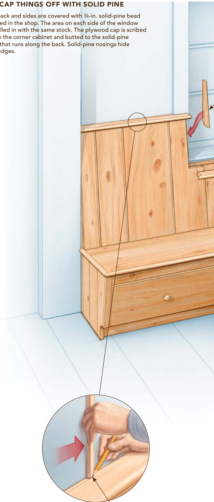
Scribe caps to wall for a consistent overhang.
