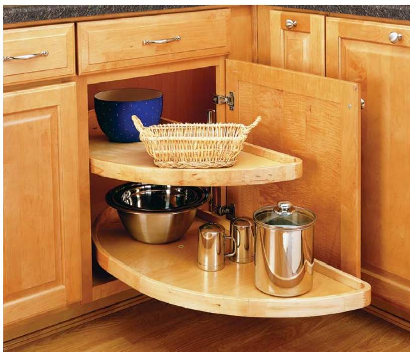
CURVING AROUND A CORNER. Rev-A-Shelf's Half Moon shelves pivot and pull out of a blind corner. The 5/8-in.-thick multi-ply wood trays come sized for door openings as small as 12 in. and can be used in framed or frameless cabinets.
