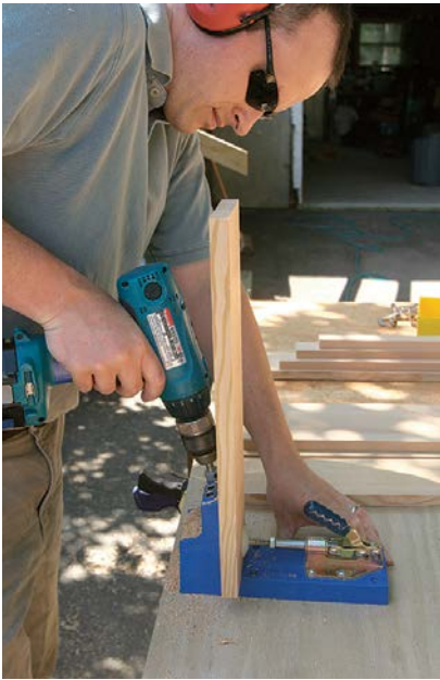
A POCKET-HOLE JIG MAKES ASSEMBLY EASY. Drill two pocket holes in the end of each rail and each inner stile.
