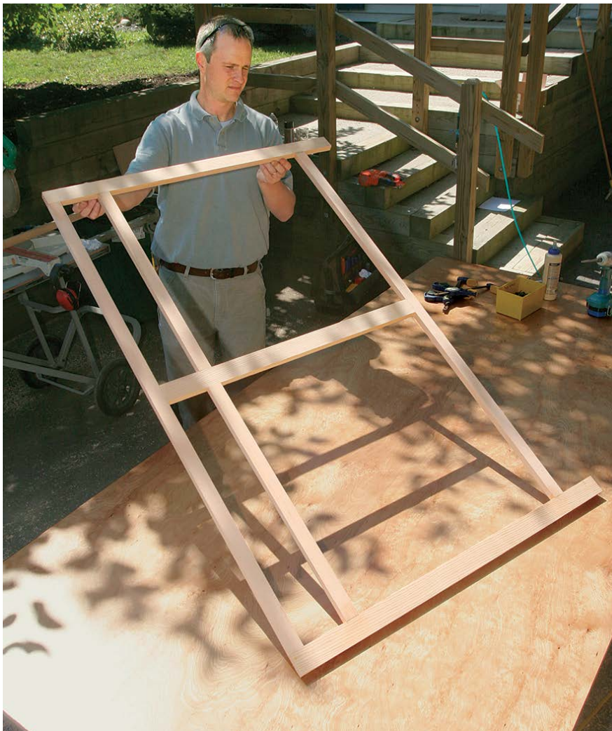
A POCKET-HOLE JIG MAKES ASSEMBLY EASY. Drill two pocket holes in the end of each rail and each inner stile.
