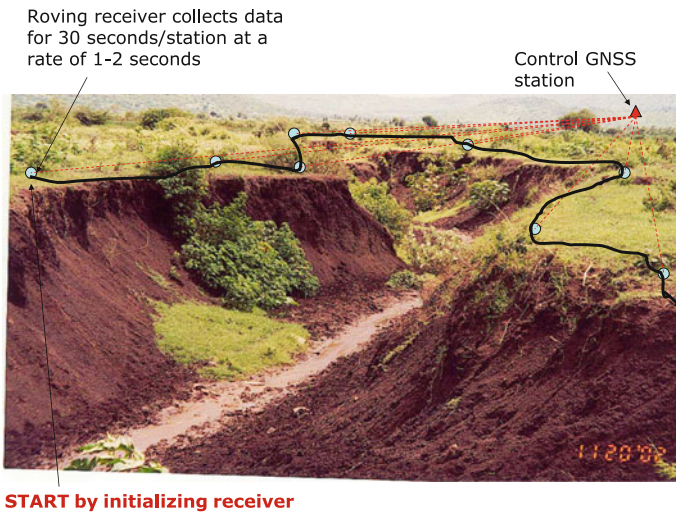
Fig. 9.10 Monitoring of the extent of erosion using the stop-and-go positioning method. The triangle indicate the control station while the circles indicate the positions occupied by the roving receiver. Initialization has to be done at the first station and a lock on four or more common satellites maintained
