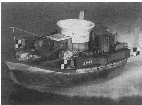
Fig. 1.9 SR.N1 – the first British ACV, which successfully crossed the English Channel.
