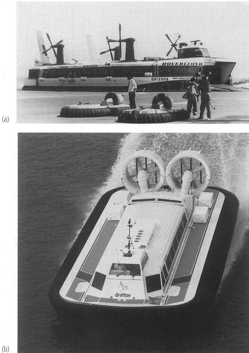
Fig. 15.1 Air propulsion types. (a) Pylon mounted open propellers on Hoverlloyd SRN-4 at Calais. The two integrated ducted fan craft in the foreground had just crossed the channel on the 25 th anniversary of the first crossing by SRN-1. (b) Twin ducted propellers in the Griffon 2500TD.
