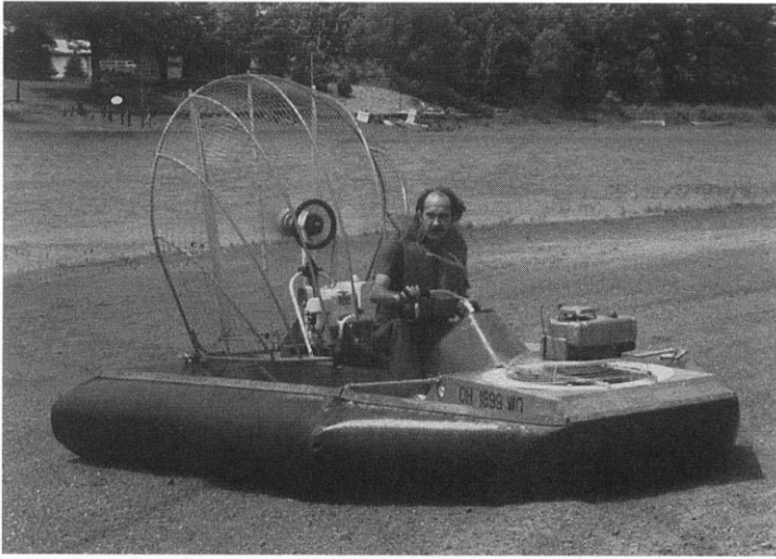
Fig. 15.8 View of a small craft with large two-blade propeller, the Universal Hovercraft UH-15P.
