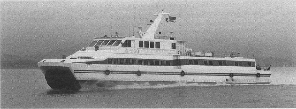
Fig. 1.41 70 seat/sleeping berth, 2 tonne cargo, steel hull, 33 knot SES, delivered for service August 1995.
