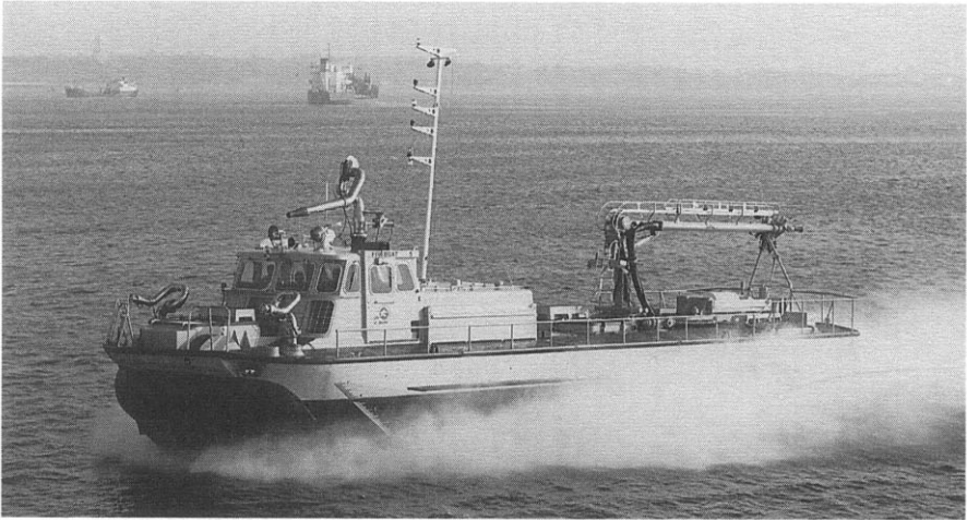
Fig. 1.18 Hovermarine HM-221 SES fireboat on trials before delivery to port of Tacoma.
