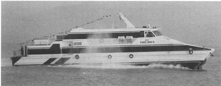
Fig. 1.40 200 seat, 32 knot passenger SES built in GRP, delivered for service December 1995.
