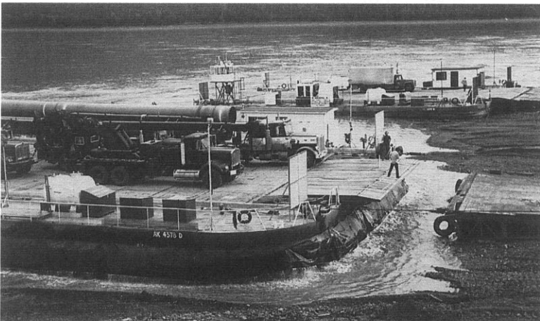
Fig. 15.4 Air cushion platform propulsion. (a) Direct propulsion by hydraulic powered wheels/tracks on the Wartsila Vector. (b) Winch propulsion along wires across the Peace river in Alaska during pipeline construction.
