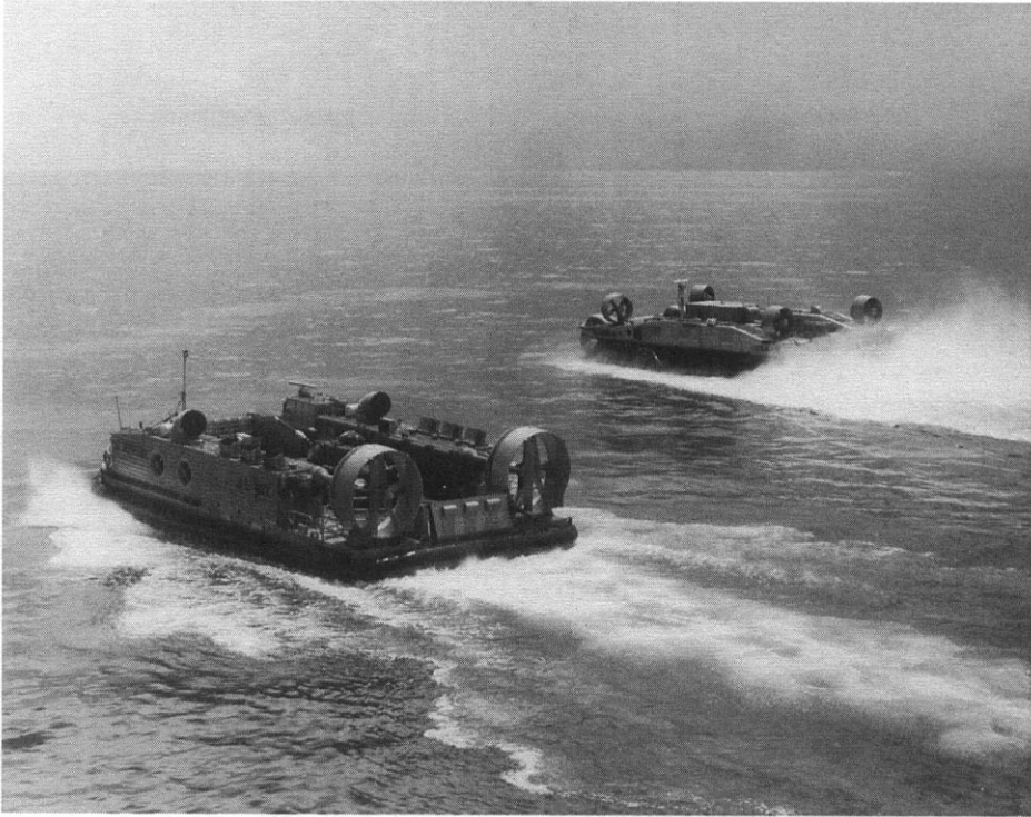
Fig. 16.14 Bell Textron Jeff (B) Showing two sets of 3 TF40 gas turbines driving lift fans and bow thrusters forward, and ducted propellers at the stern. Aerojet General Jeff (A) is in the background.
