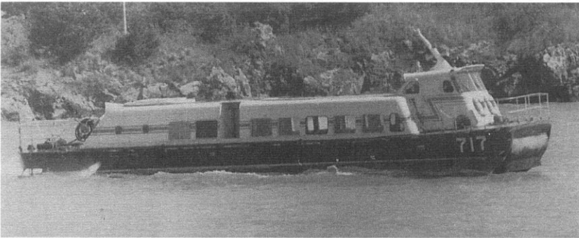
Fig. 1.33 First Chinese water-jet propelled passenger SES series 717.
