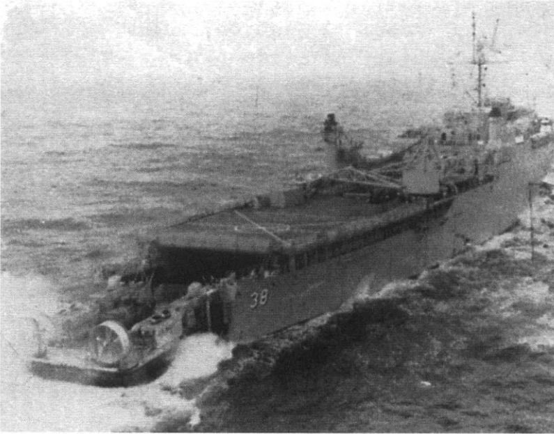
Fig. 6.1 US LCAC-001 entering into the landing ship Pensacola .
