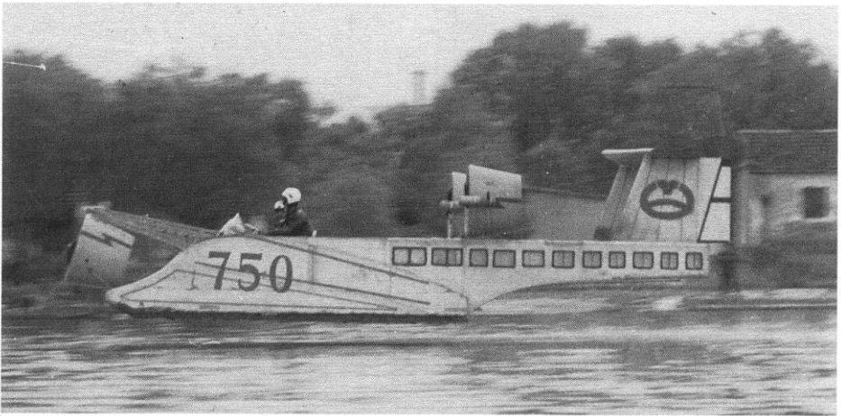
Fig. 1.7 First Chinese power augmented wing in ground effect craft model 750.
