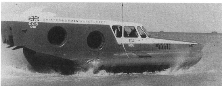
Fig. 15.12 The Cushioncraft CC5 – a very quiet centrifugal fan propelled craft.
