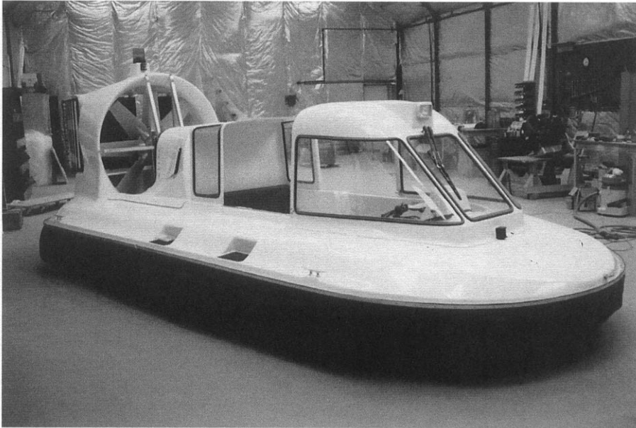
Fig. 16.6 Small craft integrated lift/propulsion from single ducted fan with horizontal splitter plate.
