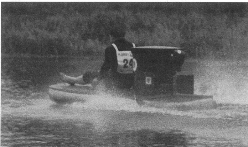
Fig. 15.1 (c) Integrated lift/thrust from single axial fan on the Griffon 375TD. (d) Air jet propulsion on an 'amateur' hovercraft racing in 1967.
