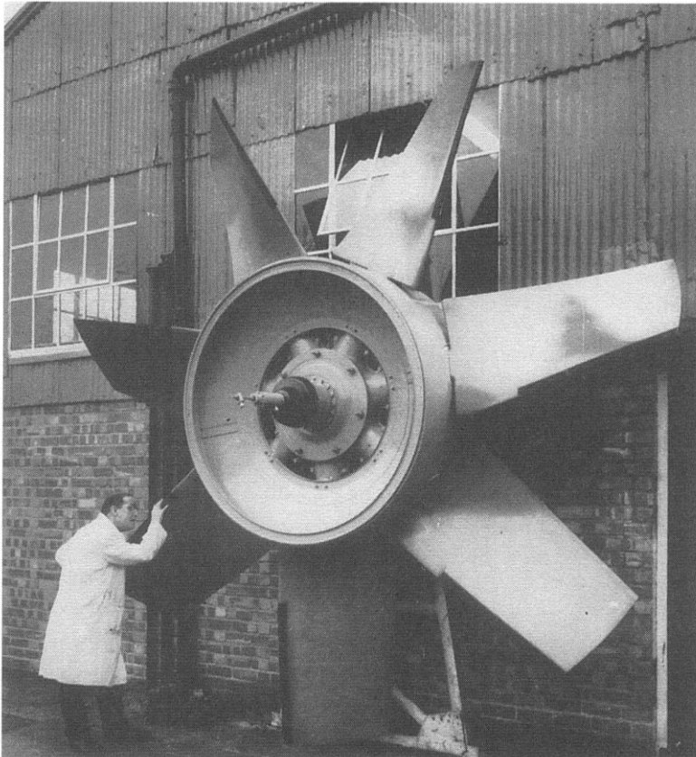
Fig. 15.17(b) The Dowty T2 ducted fan impeller.
