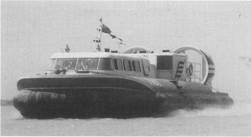
Fig. 1.37 Diesel engine propulsion ACV design 716-II.
