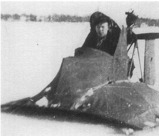
Fig. 1.2 Finnish ACV constructed by Toivio Kaario in 1935.
