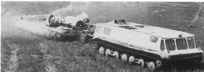
Fig. 6.6 Ground wheels for the guidance of air cushion platform.
