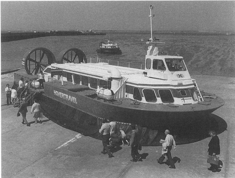
Fig. 15.13 A rotating thruster unit (AP1.88).
