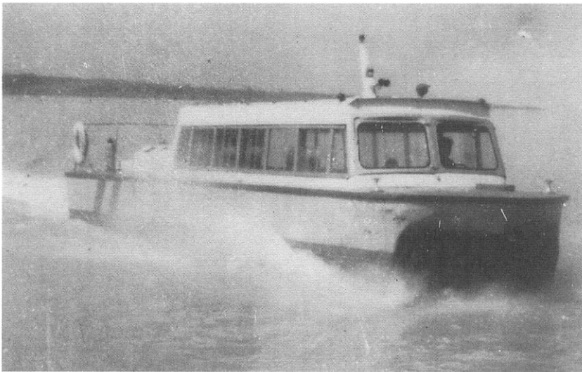
Fig. 1.38 Passenger SES design WD-901 with single water-jet propulsion unit.
