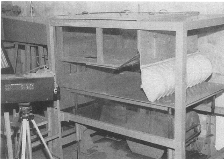
Fig. 2.6 MARIC's small skirt test rig.
