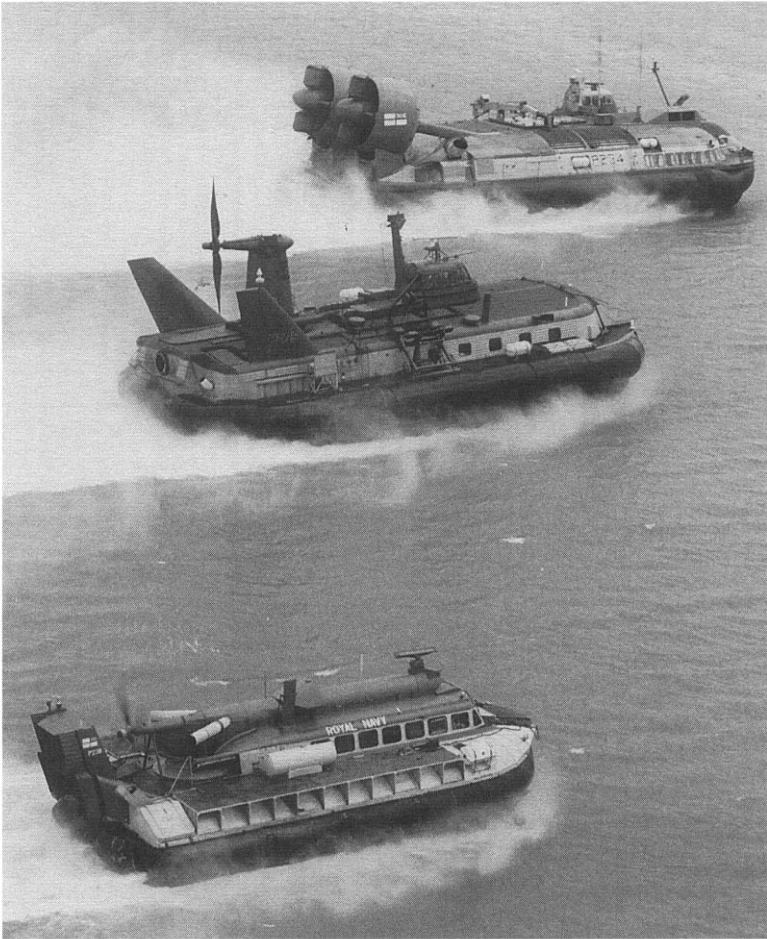
Fig. 1.13 British military ACVs from the 1970s, SR.N6, BH.7 and VT.2, in formation on the Solent.
