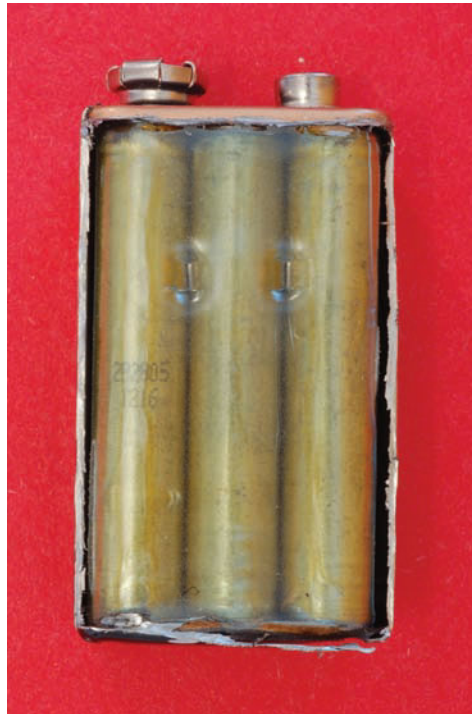
FIGURE 13-12 Internal makeup of a 9-V battery.
