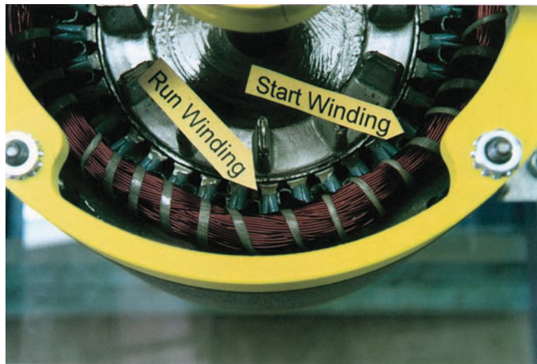
FIGURE 34-2B Stator winding of a capacitor-start capacitor-run motor. The wire size is the same for both start and run windings.
