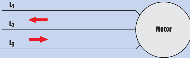
FIGURE 11-15 Current flows from line 3 to line 2.
