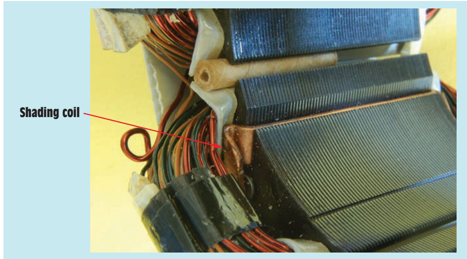
FIGURE 34-35 The shading coil is a large copper conductor wound around one side of the pole piece.
