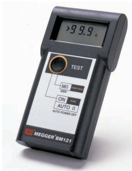
FIGURE 11-22 Battery-operated MEGGER®. (Courtesy of Megger®)
