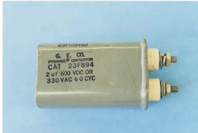
FIGURE 20-18 Oil-filled paper capacitor.
