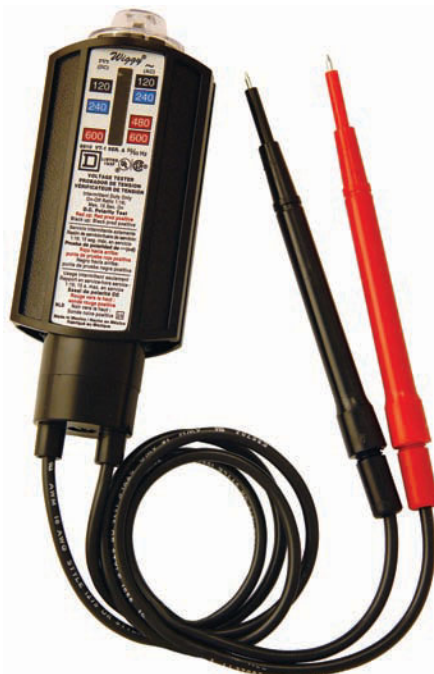
FIGURE 10-45 Wiggy® voltage tester. (Photo courtesy of Square D Company)
