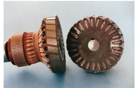
FIGURE 30-16B Cutaway view of an armature.
