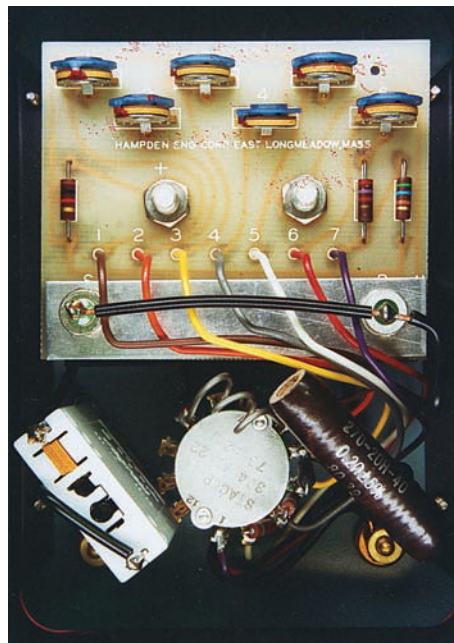
FIGURE 10-23 DC ammeter with an Ayrton shunt.
