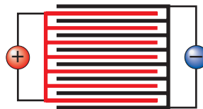
FIGURE 13-22 Multiple plates increase the surface area and the amount of current the cell can produce.
