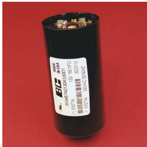
FIGURE 20-26 An AC electrolytic capacitor.
