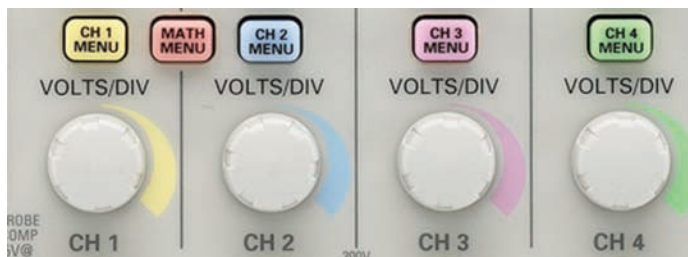
FIGURE 10-48 Voltage control knobs of a four channel digital oscilloscope. (Courtesy of Tektronix, Inc.)
