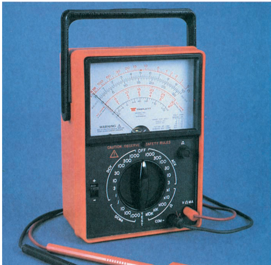
FIGURE 10-6 Volt-ohm-milliamperemeter with multirange selection. (Courtesy of Tripplett Corp.)
