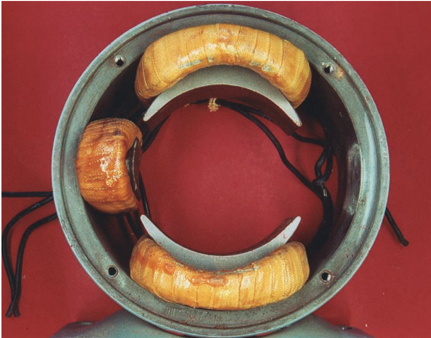
FIGURE 30-24 A two-pole DC machine with one interpole.
