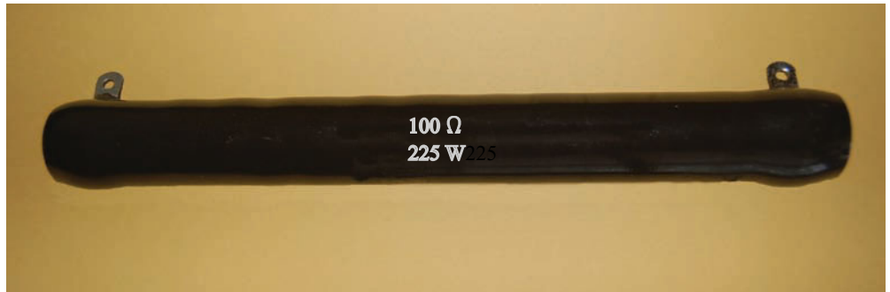
FIGURE 5-7 Wire-wound resistor with hollow core.
