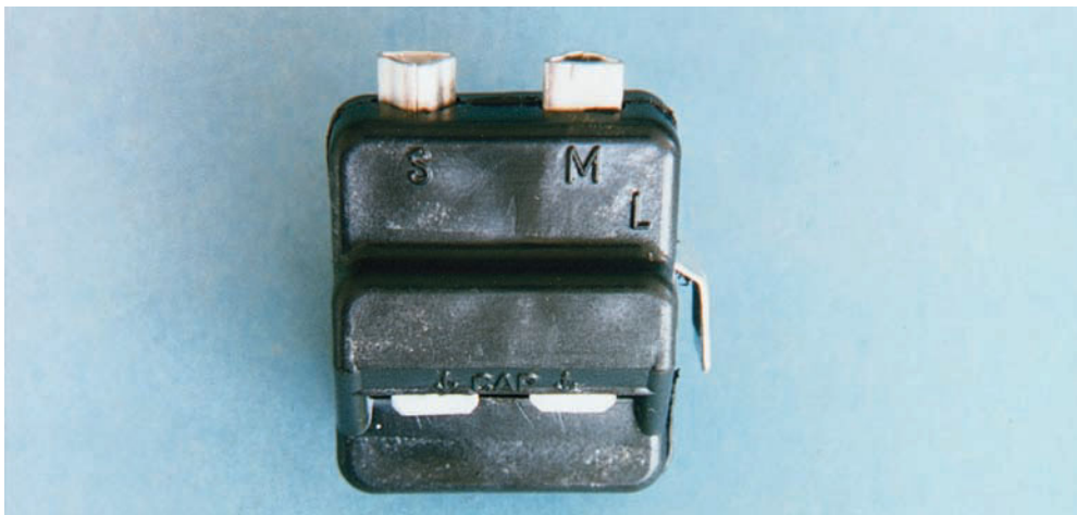
FIGURE 34-12 Solid-state starting relay.
