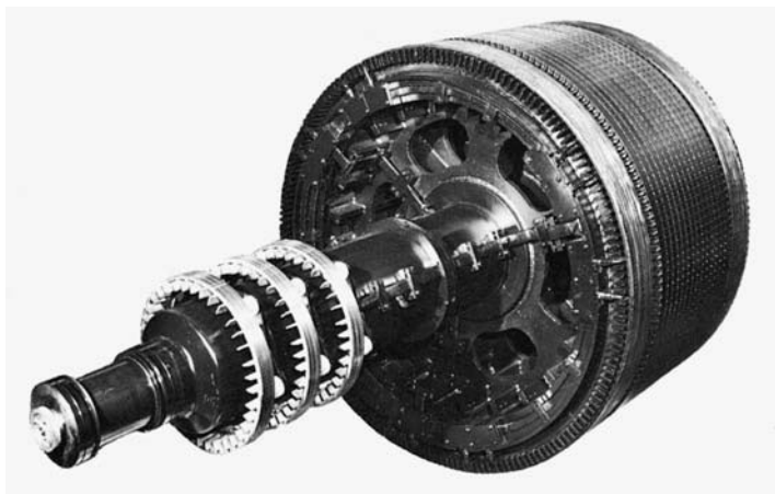
FIGURE 33-46 Rotor of a wound-rotor induction motor.
