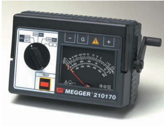
FIGURE 11-21 A hand-crank MEGGER®. (Courtesy of Megger®)
