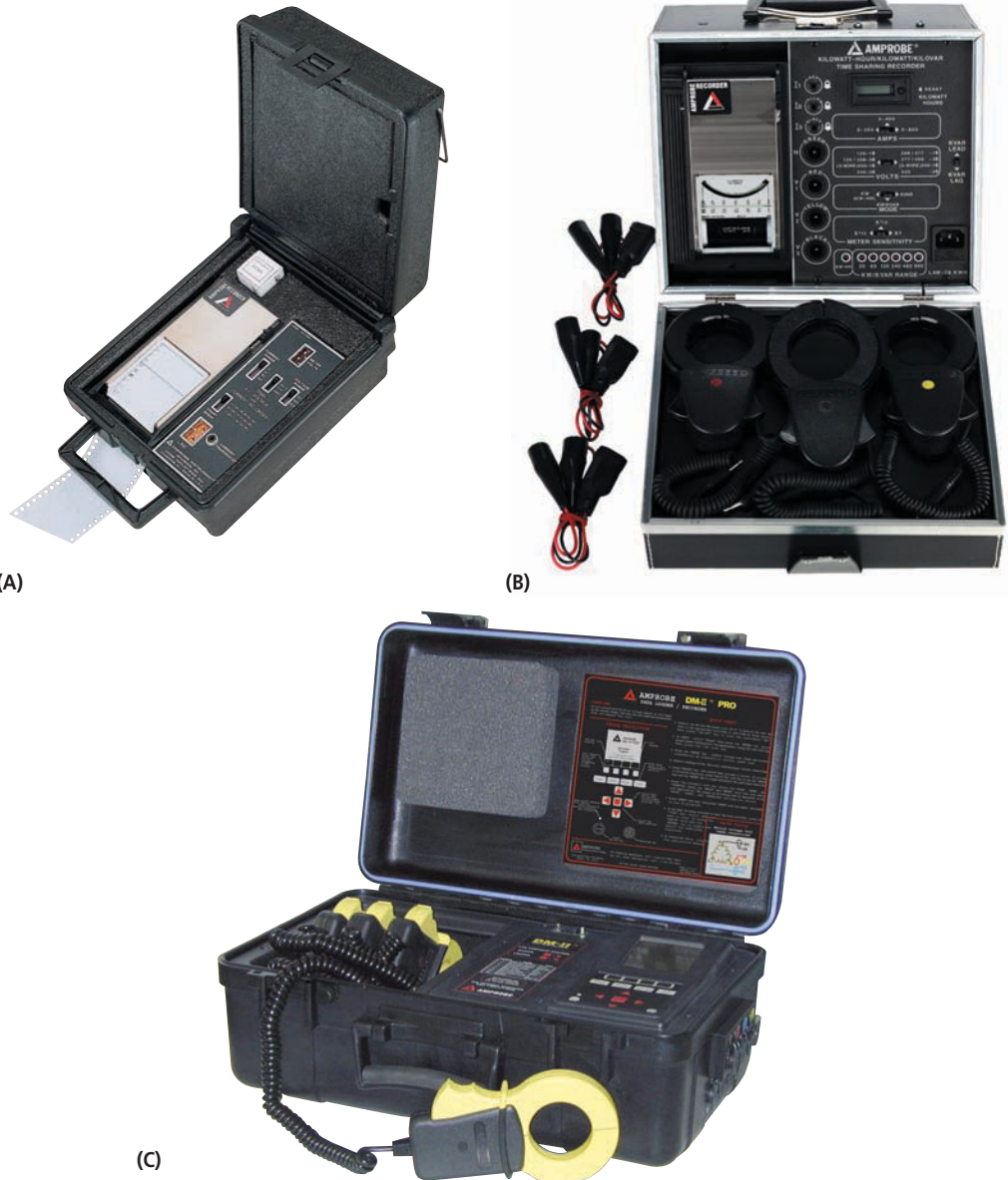
FIGURE 10-63 (A) Single-line-line recording volt-ammeter. (B) A kilowatt-kiloVAR recording meter. (C) A single-phase or three-phase voltage and current recording meter. (Courtesy of Advanced Test Products)
