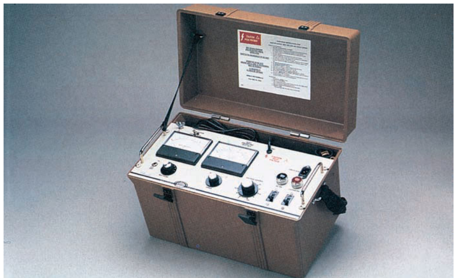
FIGURE 20-36 A dielectric test set. (Courtesy of Megger®)
