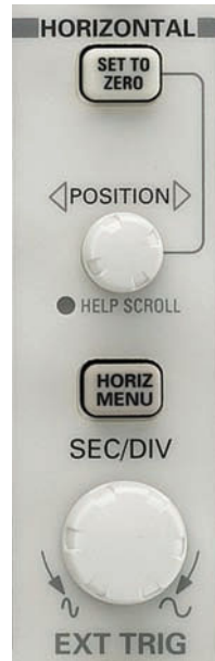
FIGURE 10-54 Time base control for a typical digital oscilloscope. (Courtesy of Tektronix, Inc.)
