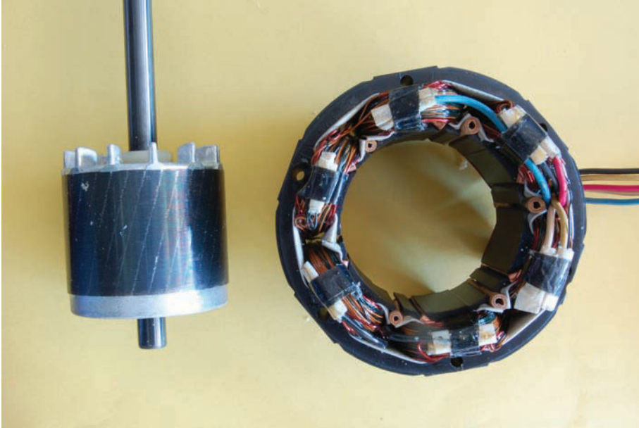
FIGURE 34-37 Stator winding and rotor of a shaded-pole induction motor.
