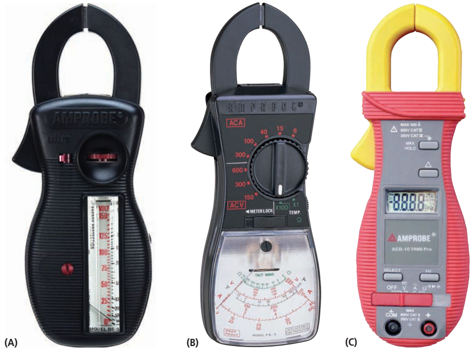
FIGURE 10-29 (A) Analog type clamp-on ammeter with vertical scale. (B) Analog type clamp-on ammeter with flat scale. (C) Clamp-on ammeter with digital scale. (Courtesy of Advanced Test Products)
