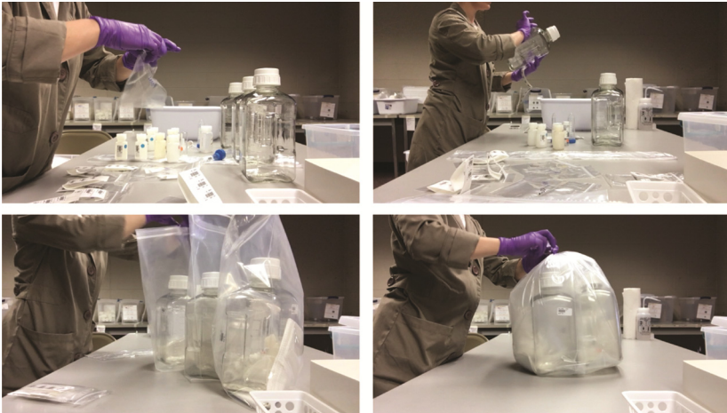
Fig. 3. An ECRL technician demonstrates the kit assembly protocol adapted for use in the FACHEP field station housed in a former elementary school. Assembly tasks for a “circle” kit include arranging the materials on a sterilized assembly table (upper left); labeling sample containers with their barcode labels (upper right); dividing the materials into three separate location sets (lower left); and finally packing the sets and the barcode label pack into a complete kit (lower right).
