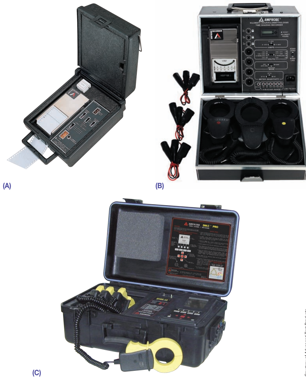
FIGURE 10-63 (A) Single-line recording volt-ammeter. (B) A kilowatt-kiloVAR recording meter. (C) A single-phase or three-phase voltage and current recording meter.
