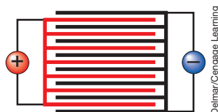
FIGURE 13-22 Multiple plates increase the surface area and the amount of current the cell can produce.
