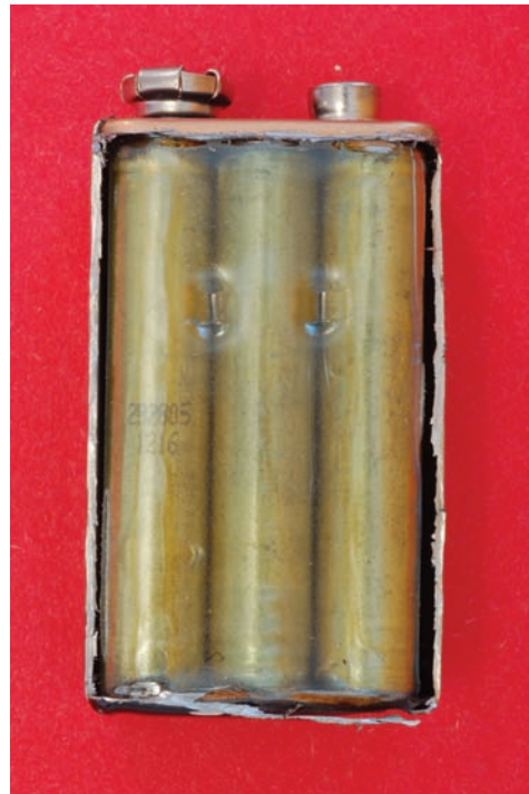
FIGURE 13-12 Internal makeup of a 9-V battery.
