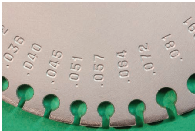
FIGURE 11-4 The other side of the wire gauge lists the diameter of the wire in thousandths of an inch.
