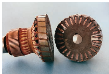
FIGURE 30-16B Cutaway view of an armature.
