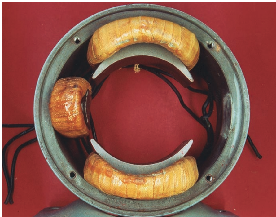
FIGURE 30-24 A two-pole DC machine with one interpole.
