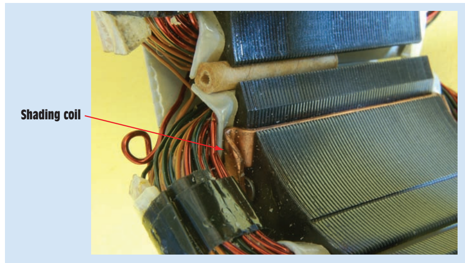
FIGURE 34–35 The shading coil is a large copper conductor wound around one side of the pole piece.
