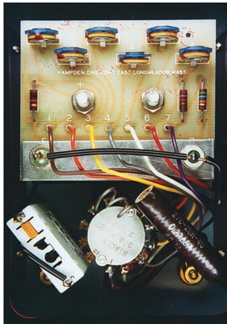
FIGURE 10-23 DC ammeter with an Ayrton shunt.
