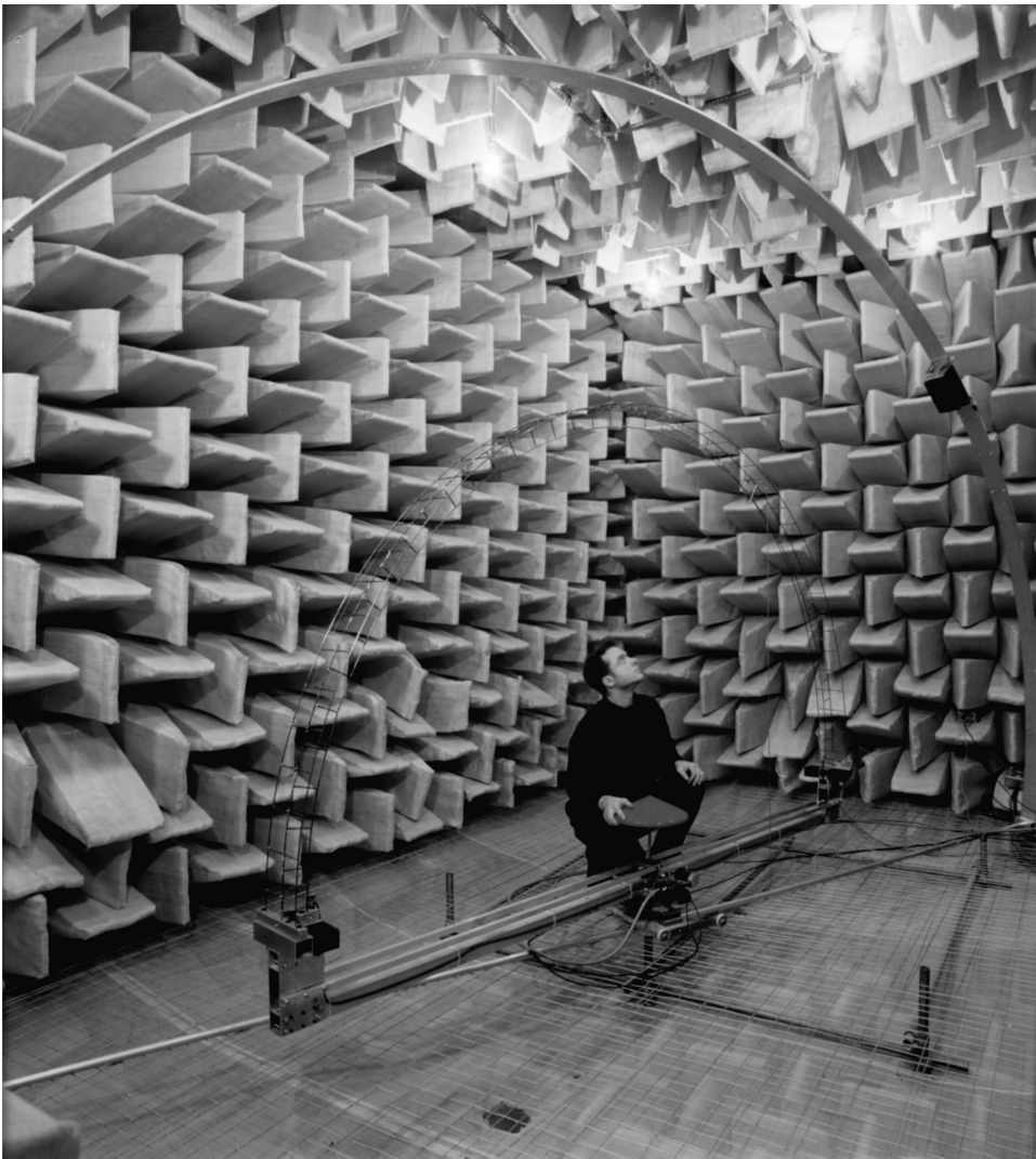
Figure 5.5 A system for measuring the scattering from a surface over a hemisphere. The diffuser being tested is the small pyramid in the centre. The source arc is most obvious; the receiver arc is acoustically transparent and is thus more difficult to see. (Reproduced from AES-4id-2001, J. Audio Eng. Soc. , 49, 149–165, 2001, with permission from the Audio Engineering Society.)
