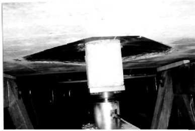
(a) S4: Failure around plate perimeter
