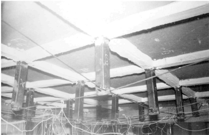
Figure 2 Parabolic cable network
