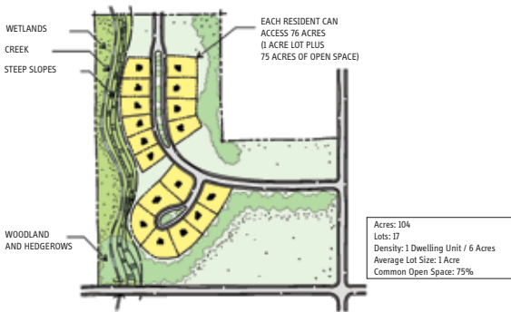
A comparison of land use in a typical suburban development (top) and a cluster development.
