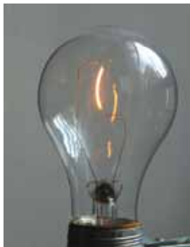
The filaments of a toaster and an incandescent bulb work in exactly the same way, which explains the wasted heat emitted by the bulb.
