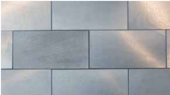
These aluminum tiles are made from 100 percent postconsumer aluminum sourced from reclaimed aircraft parts.
