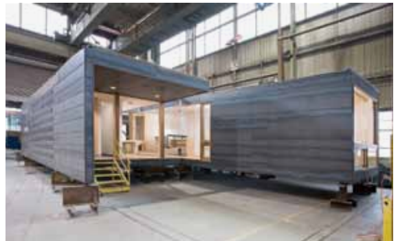
Koby Cottage (2009), designed by Garrison Architects, is a contemporary example of a prefab home (shown in factory).
