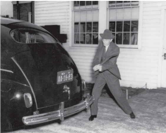
Henry Ford was enamored with bioplastics. Here he is demonstrating that the bioplastic trunk of his car can resist a blow from an axe.
