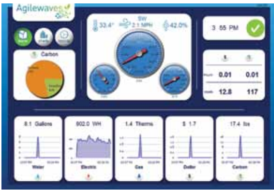
“Smart panels,” or “building dashboards,” allow monitoring of building performance, including electricity, gas, and water consumption.
