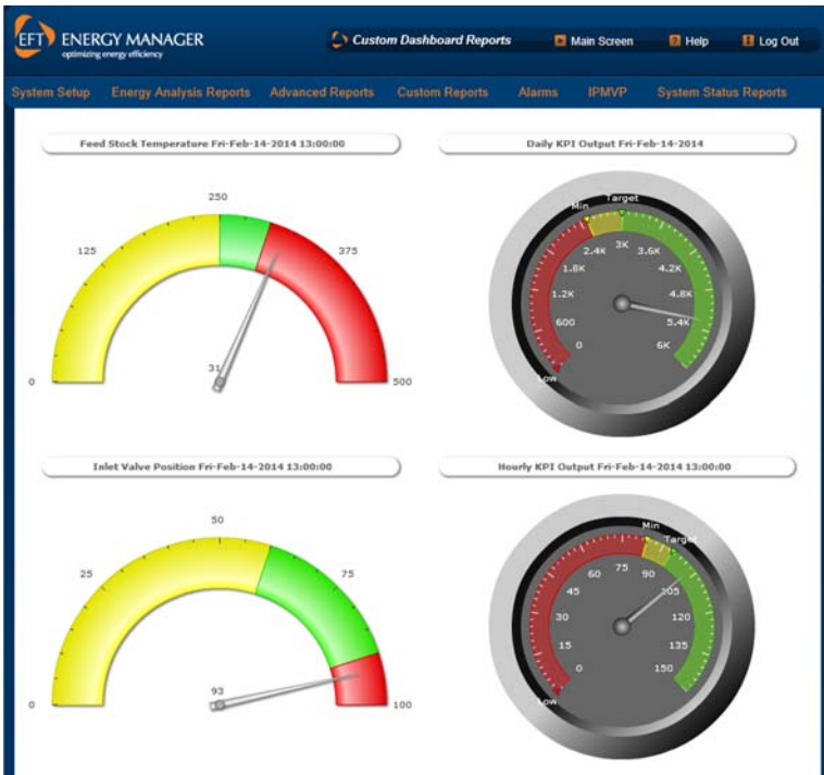
Figure 27.2. A simple dashboard created specifically for a line operator. It shows both EnPIs and the status of variables under his/her control.
