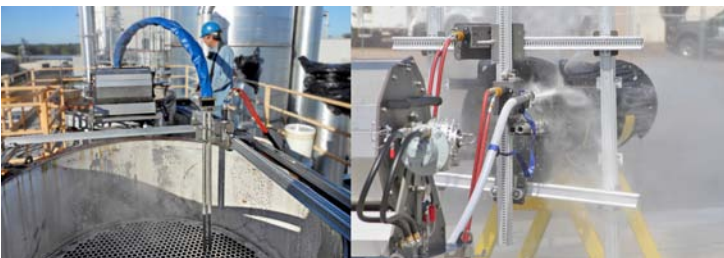
Figure 11.2. Equipment for clean in place (CIP) applications. (Source: Photos courtesy of StoneAge Inc.)
