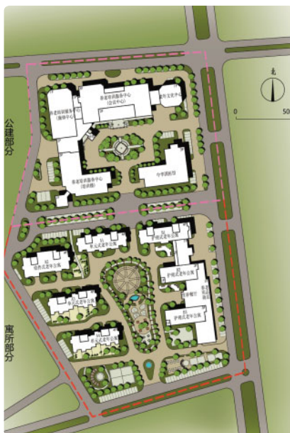
below: Site plan showing the arrangement of public facilities and hospital in the northern portion of the site and the private residential areas divided into private accommodation (lower west portion) and the care home (lower east).
