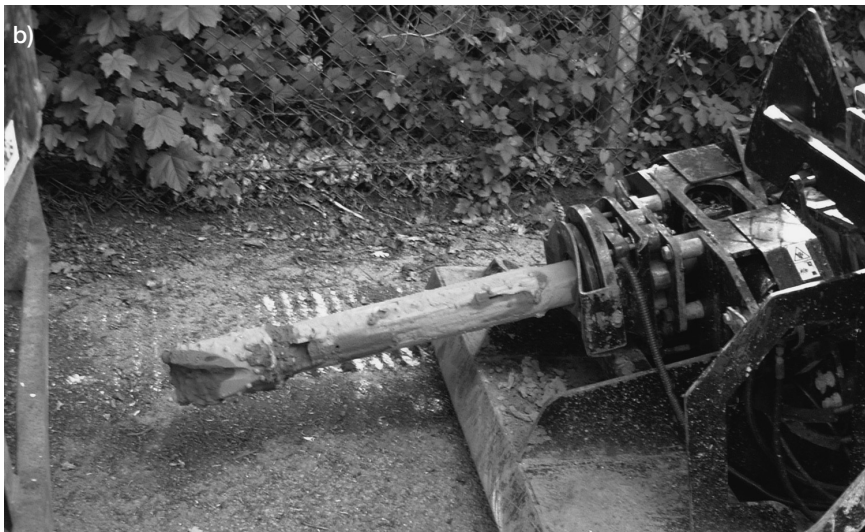
Figure 5.85 a) An example of an HDD rig (note an example of a ‘reaming’ device beside the rig on the left), b) a close-up of the pilot drill head (note the ‘chisel’ type drill head with an angled face)
