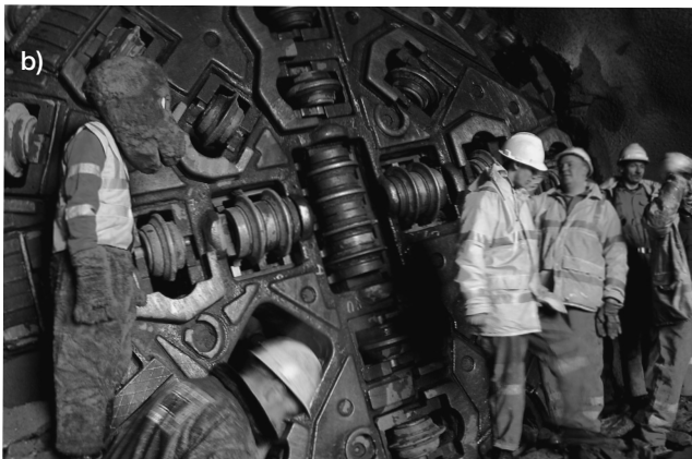
Figure 5.18 a) and b) 5.03 m diameter Herrenknecht S-351 Gripper TBM used at Glendoe, UK (courtesy of Herrenknecht)
