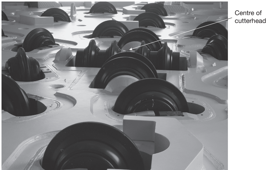
Figure 5.21 An example of some hard rock disc cutters (as used in granite). Note the arrangement of the cutters as one moves from the centre of the cutterhead to ensure all the face is excavated (courtesy of Herrenknecht)
