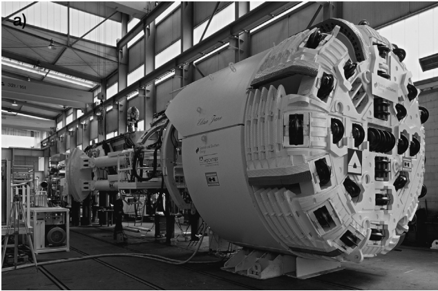
Figure 5.17 Gripper machine with multiple 'X' formation gripper shoes (diameter 8.8 m, length 5.7 km, through Gneiss in Quinling China) (courtesy of Aker Wirth)
