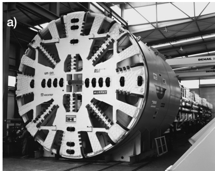
Figure 5.27 8.160 m diameter, 100 m long Herrenknecht S-192 Mixshield TBM used on the Channel Tunnel Rail Link (CTRL) project in the UK, a) before and b) at breakthrough. This machine drove through alluvium, chalk and flints (courtesy of Herrenknecht)
