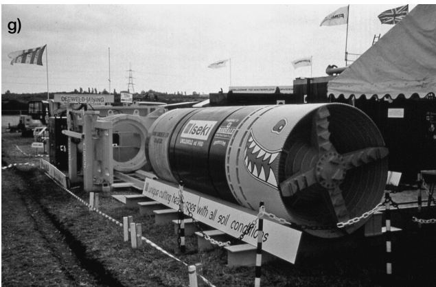
Figure 5.83 (continued) e) control panel for a micro- tunnelling machine, f) and g) examples of microtunnelling machines
