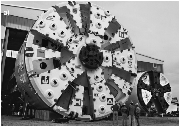
Figure 5.28 14.2 m diameter Herrenknecht S-108 Mixshield TBM used to construct the 4th Elbe Tunnel in Hamburg, Germany, a) before and b) at breakthrough (length of drive 2.56 km, through sand, glacial drift, silt, gravel and boulders) (courtesy of Herrenknecht)
