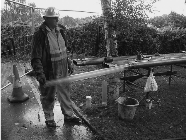
Figure 2.6 Triple core barrel sampler (double core barrel with a plastic liner) used with rotary drilling
