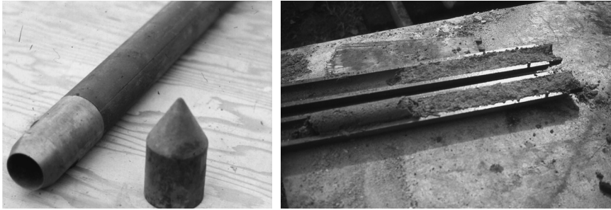
a) b) Figure 2.9 Split barrel sampler used for the standard penetration test: a) the open tube is used for fine grained soils and the cone for coarse grained soils and b) in fine grained soils a sample can be obtained for visual inspection (courtesy of Dr Ron Jones)
