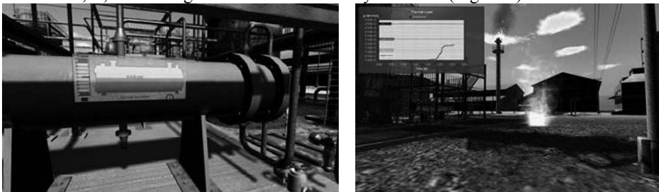
Figure 3: Two examples of AVR showing variables from the process simulator (left, reboiler level and corresponding alarms) and from the accident simulator (right, thermal load with I, II, and III degree burns).
