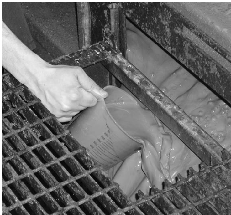
Figure 4.1. Sample is taken directly from the effluent stream.
