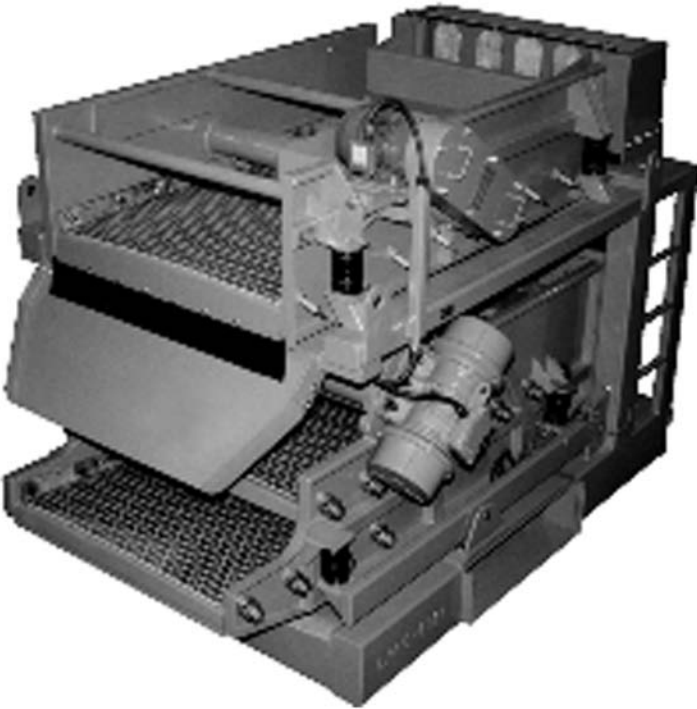
Figure 7.19. Integral cascade unit with multiple vibratory motions.
