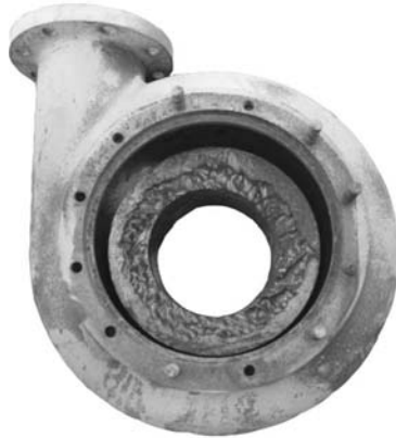
Figure 18.14. Results of abrasive fluid cavitation.
