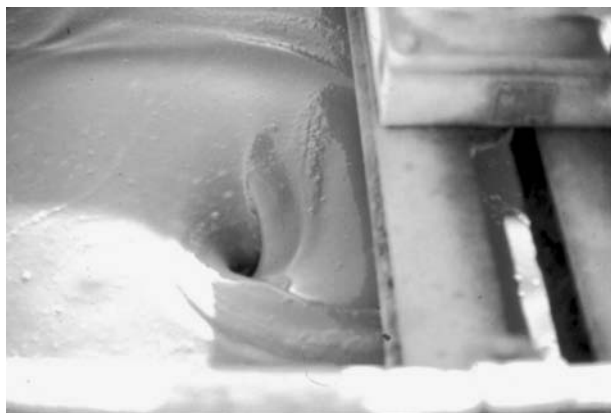
Figure 10.10. Vortex formation in fluid.
