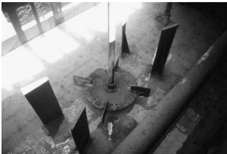
Figure 10.11. Baffles: pointed at corners; note poor placement of pipe.
