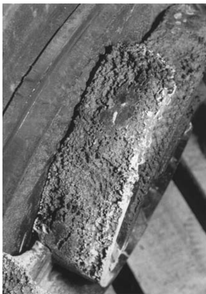
Figure 18.12. Results of clear fluid cavitation.
