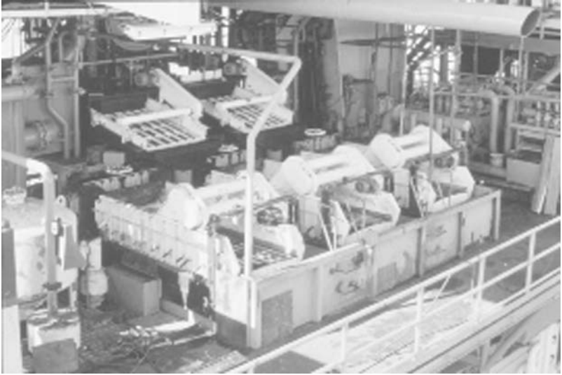
Figure 7.18. Separate unit cascade system.
