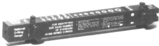
Figure 3-10. O-ring diameter may be measured on an o-ring gauge.
