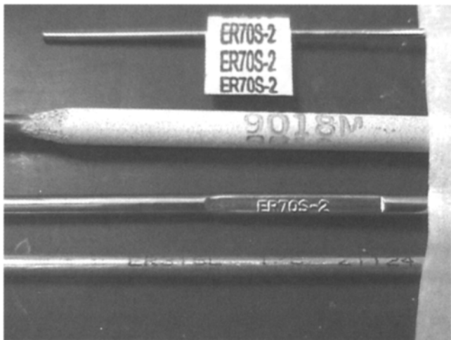
Figure 6-13. Welding filler metals are identified by a stenciled AWS designation at the end of a coated electrode and a paper flag at the end of bare wire.
