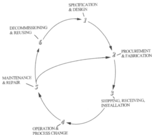
Figure 1-1. Individual job functions come into play at every step of the materials lifecycle.
