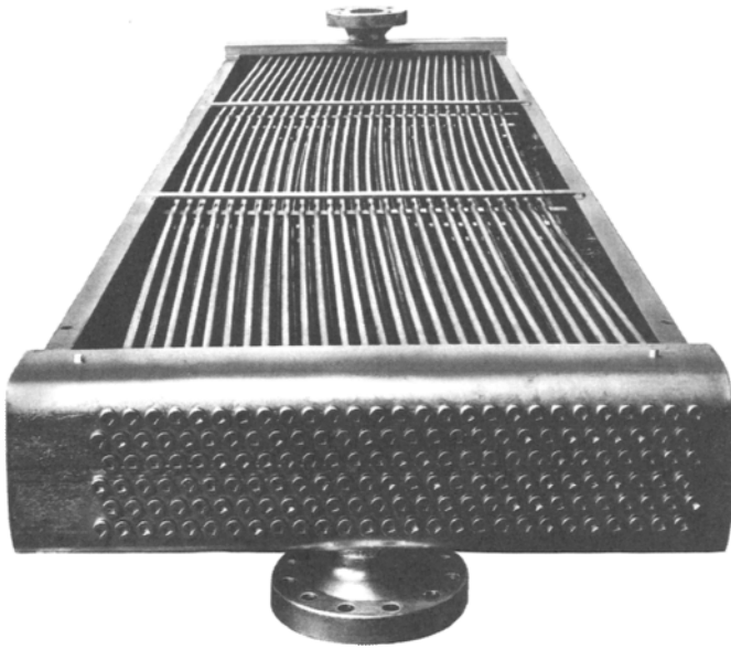
Figure 10-6. Open tube sections. (Used by permission: Griscom-Russell Co./Ecolaire Corp., Easton, PA.)
