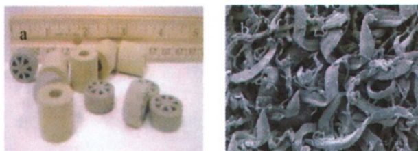
Plate 6.1. a) Conventional catalyst pellets b) Scanning electron micrographs of FeCrAlY felt substrate used in microchannel reactor.
