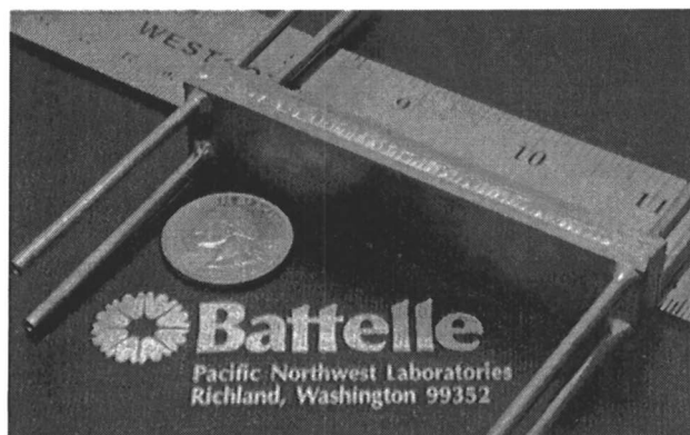
Figure 4. Example of 20-W integrated methanol steam reformer, containing catalytic combustor, vaporizers, recuperators, and catalytic steam reformer.
