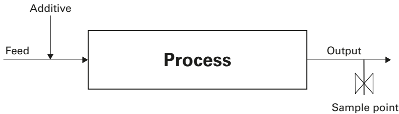
Figure 5.1 Chemical injection and sampling process
