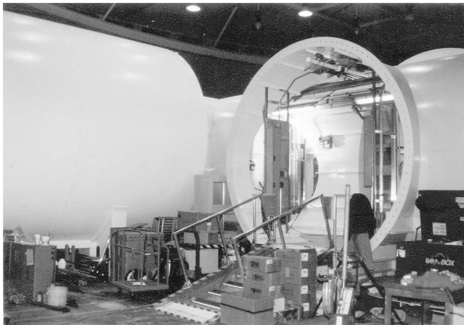
FIGURE 2 Rocket body simulating crew quarters for Mars.
